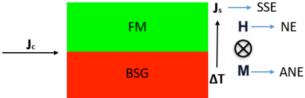
Figure 1-1.6.2: The thermal gradient generated across the thicknesses of the bilayer. The temperature gradient is created along the thicknesses of the materials. It shows the cases of NE, ANE and SSE.
