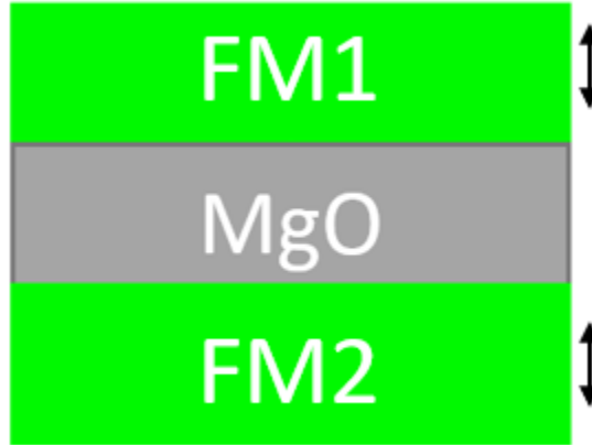
Figure 1-1.1.1: Schematic of a typical MTJ structure. The green blocks are the ferromagnetic layers. The arrows refer to the direction of magnetization.
