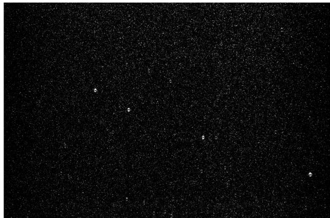
Figure 2.3: Instantaneous realization of the particle laden flow. Both the mm-sized spherical PS particles and the microscopic silver-coated glass tracer particles are visible.
