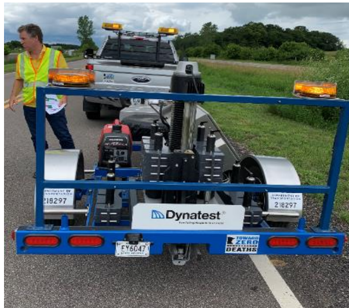
Figure 3-6: MnDOT Falling Weight Deflectometer device (Picture Courtesy: Manik Barman, 2020).
