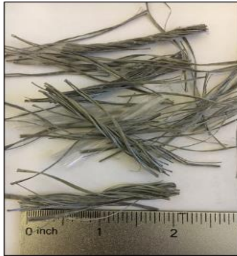
Figure 3-4: Photograph of the Forta Ferro fibers used in MnROAD 2017 FRC test cells.
