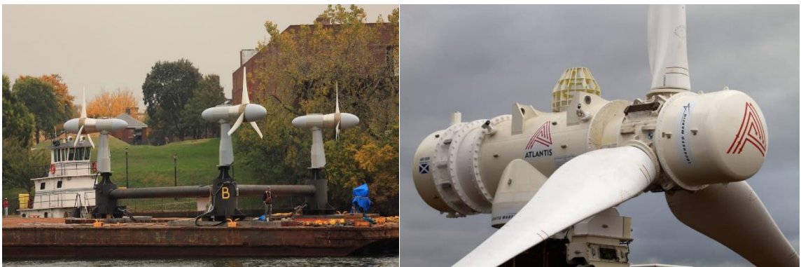
Figure 2: Gen5 System Installation at RITE Project (Left) and Atlantis Energy's AR1500 tidal turbine (Right) [23,30]
