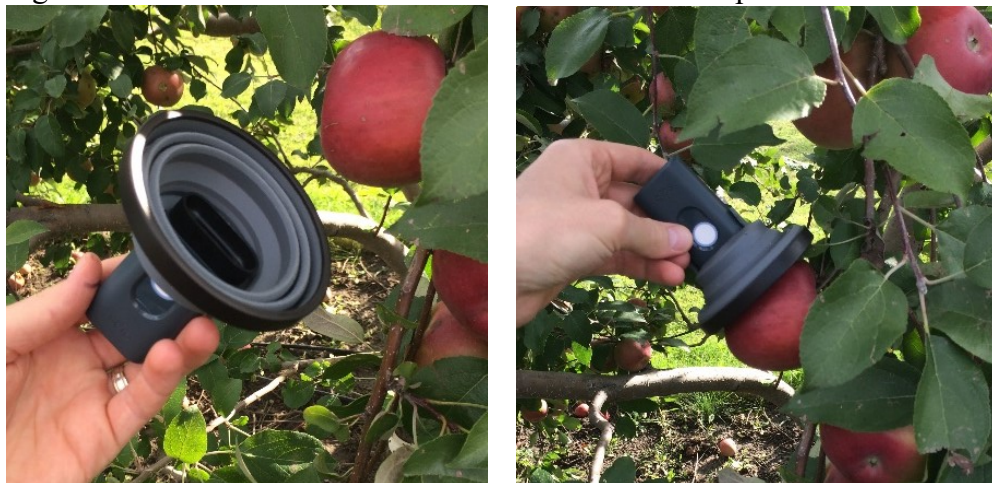
Figure D- 1. Modifications for outdoor use of the SCiO spectrometer
