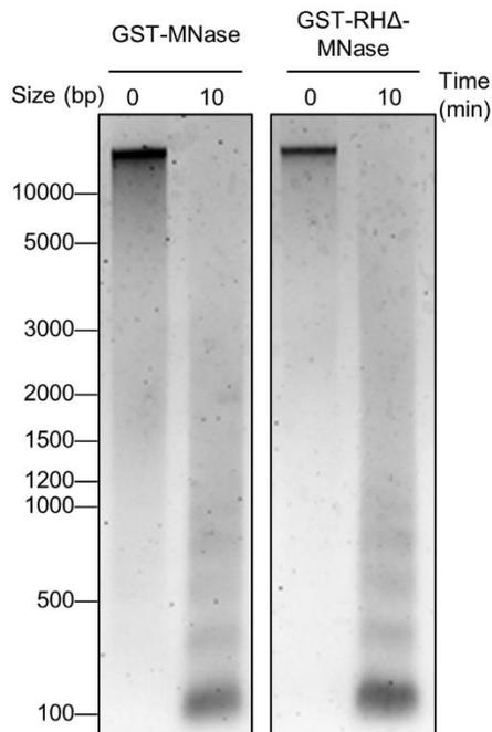
**Figure 3: Examining MNase activity of purified GST-MNase and GST-RHA-MNase proteins.** Samples were purified at different digestion time points and run together on 1% agarose gel. The gel was stained by ethidium bromide for imaging. bp, base pairs, min, minutes.
