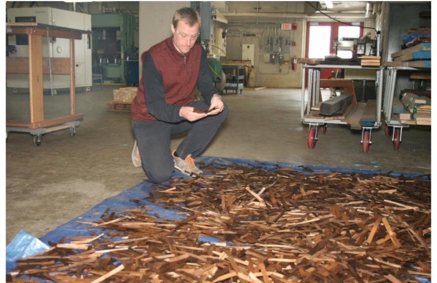
*Matt Aro inspects thermally modified wood strands before shipping to the University of Washington where it will be made into strand veneer lumber for testing. 2019 archive photo.*
