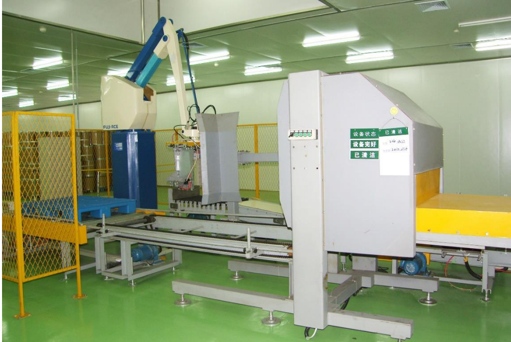
Figure A2.5. Automatic pallet packing of finished vitamin product
