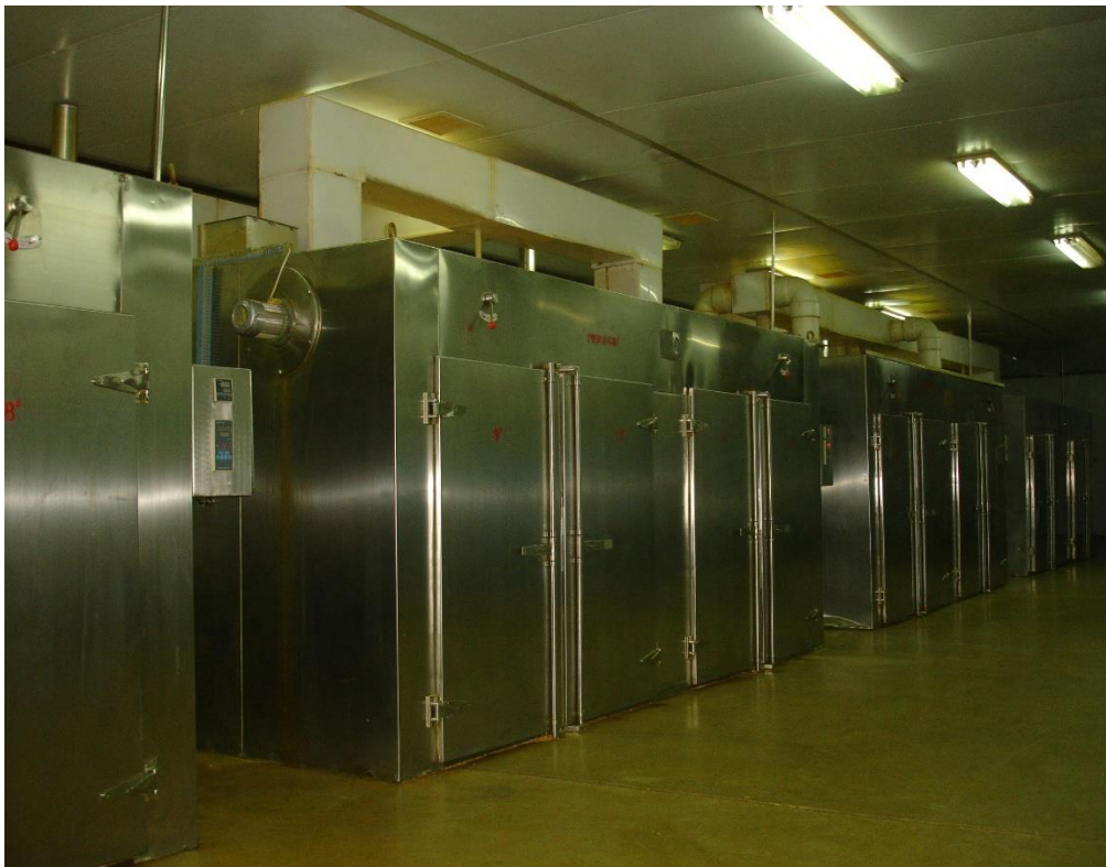
Figure A2.4. Sanitary stainless-steel vitamin product dryers
