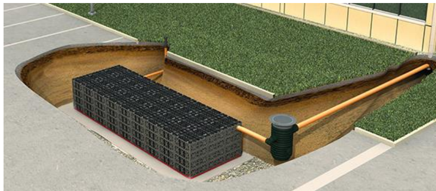
Figure 25 sustainable urban drainage system
