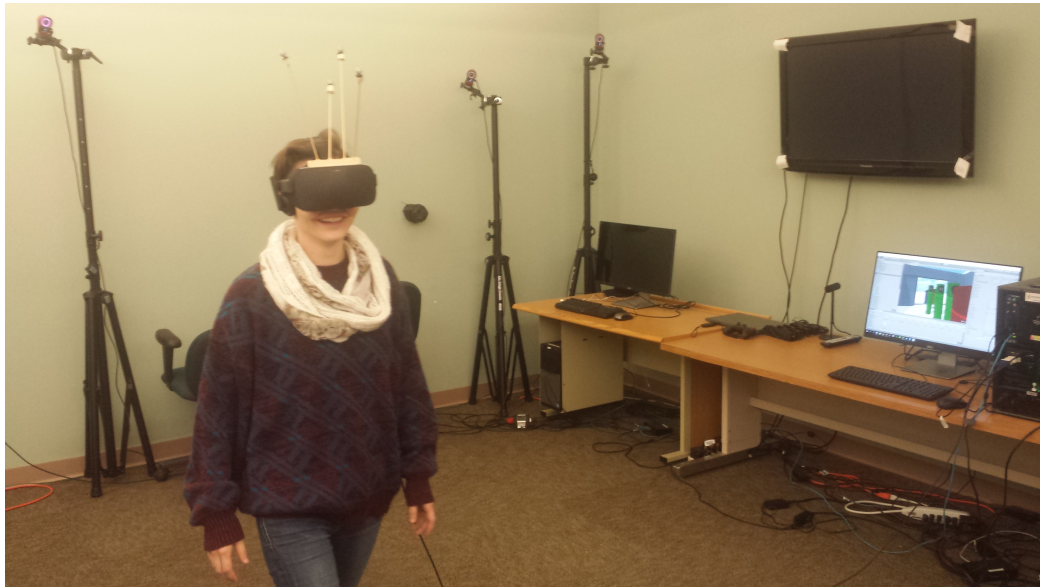
Figure 4.3: Lab Setup. A participant being tracked as she moves through the physical lab environment reacts to virtual agents in a simulated crowd.
