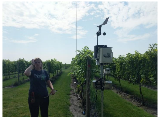
A wireless distress call speaker in a vineyard, mounted to a weather station. Photo: Davy DeKrey.
