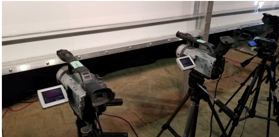
Figure 2.6.1: Picture of video cameras on tripods approximately 1 to 2 feet from the side of the flume. Spotlights behind the cameras provided the lighting needed for the videos. A white backdrop was added to prevent the cameras from focusing on background objects.
