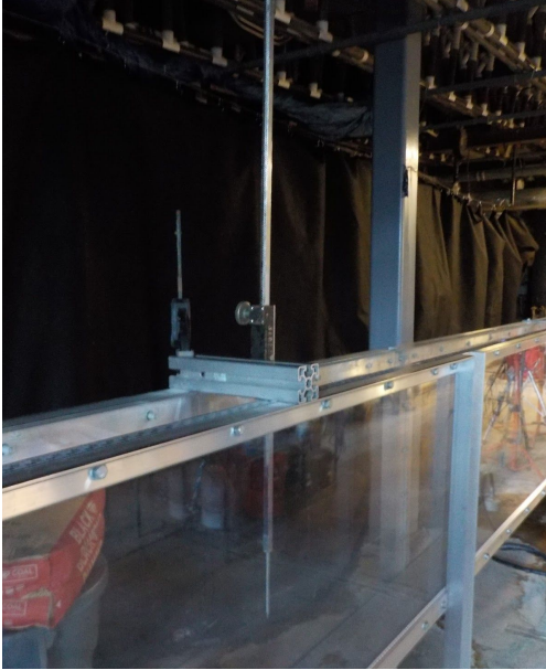
Figure 2.7.5: Photo of the point gauge used to measure the final surface of deposits attached to the top of the flume via a clamp. Point gauge measurements were taken of the entire deposit by removing the clamp and sliding the system to a new location.
