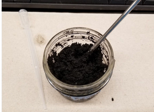
Figure 2.8.3: Picture of a sample after it had been moistened and mixed thoroughly. A dropper like the one next to the sample in the picture was used to add drops of water to the sample until it was sufficiently damp.
