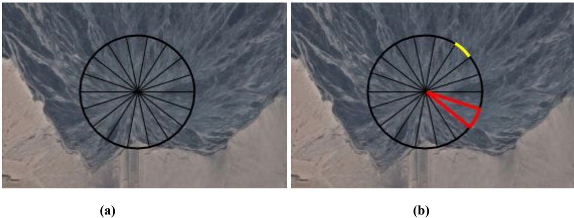
Figure 2.2.2: (a) A satellite image of a tailings delta similar to that used for this research taken on July 17, 2016. A circle with a radius of 125 meters was drawn over the estimated exit of the pipe. (b) The circle was split into 18 slices and the flow through the end of each of these slices i.e. a segment was estimated. A slice is indicated in red and the segment is indicated by the yellow.
