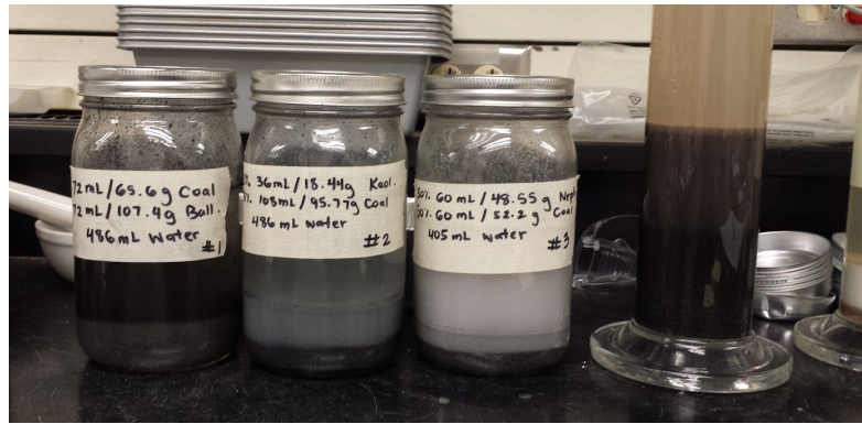
Figure 3.1.2: Picture of different mixtures tested in glass jars sitting next to a TSRU tailings sample in a settling column. Here, we wanted to see if these mixtures would form two distinct sediment layers like TSRU tailings and at similar settling rates.
