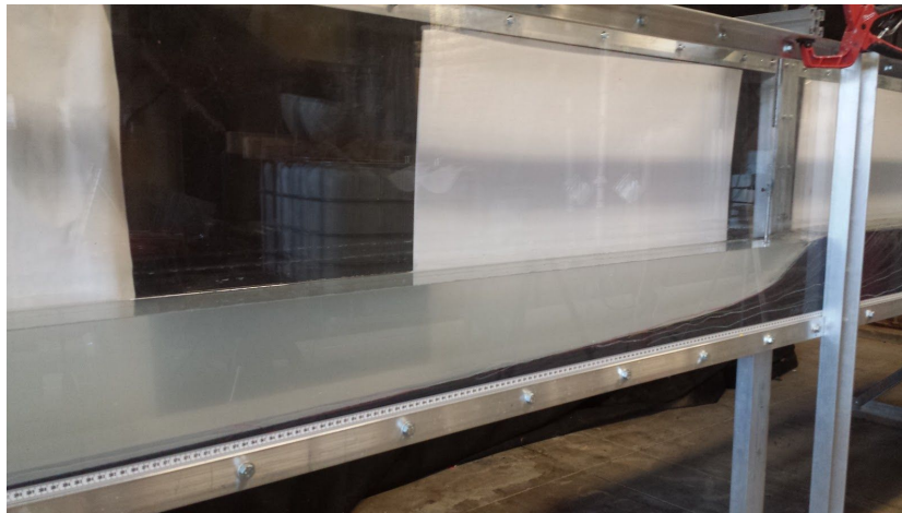
Figure 2.6.4: Picture of a deposit with a clear enough pond for surface measurements to be taken with a point gauge. The point gauge is included in the right side of the photo, attached to the top of the flume with a clamp.
