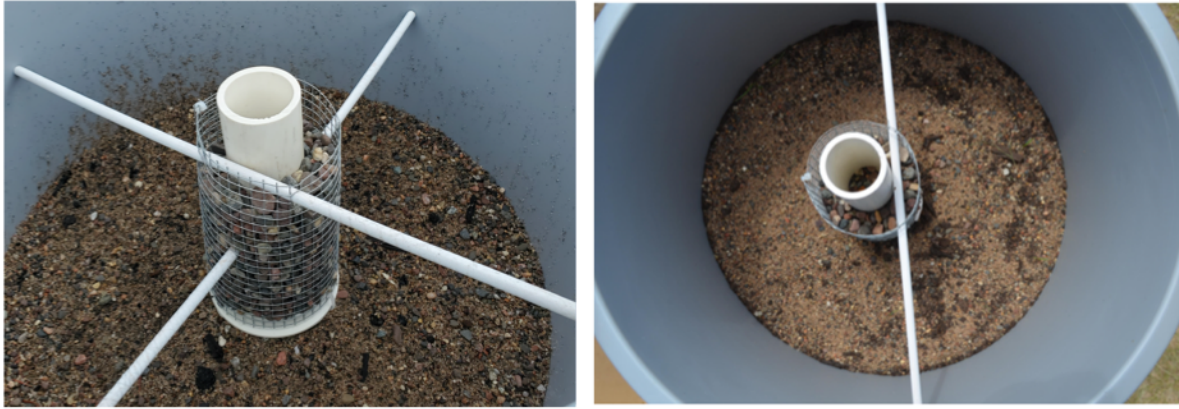
Figure 16: Side (left) and aerial (right) photos of dissipater columns.
