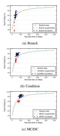
Figure 1: Percentage of faults identified compared to test suite size for generated test suites, coverage-satisfying subsets of randomly generated tests, and pure random test generation.
