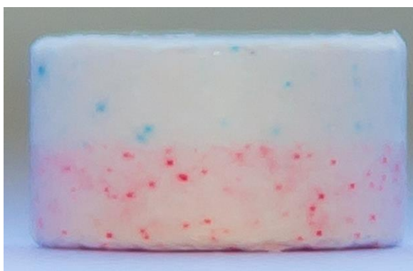
Figure 4.1 An image of a bilayer tablet (8 mm diameter). The first layer (Bottom layer) consisted of red colored MCC and uncolored lactose, while the second layer (Top layer) was composed of blue colored lactose and uncolored MCC.
