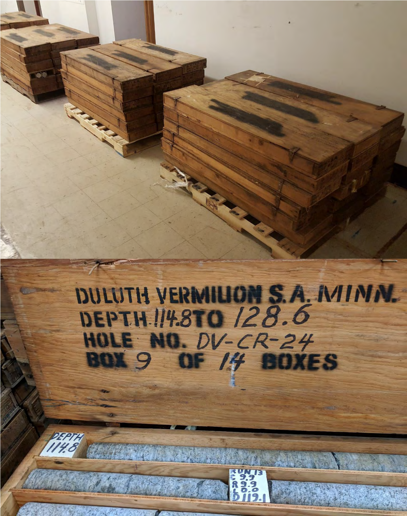
Figure 2.8 Air Force cores from Minnesota, referred to as DV Cores (Crisp, R. W. and Saucier, K. L., 1970, Tests of Rock Cores, Duluth-Vermillion Study Area, Minnesota, US Army Engineer Waterways Experiment Station, Miscellaneous Paper C-70-9)
