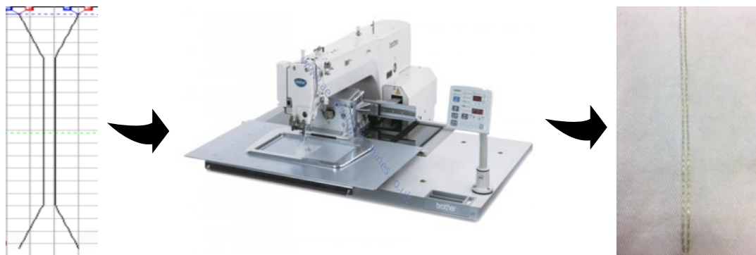
Figure 15: Stitching conductive traces using Brother BAS-342G pattern-stitching machine
