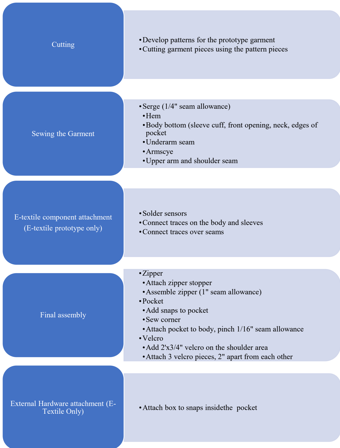
Figure 69: Steps involved in assembling both regular and e-textile thermal liners
