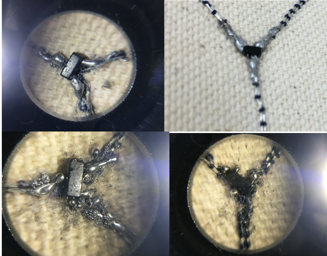
Figure 81: Example of good (top) and bad (bottom) solder joints
