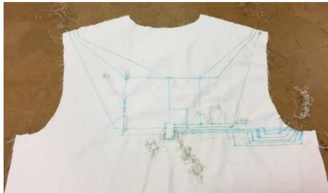
Figure 44: Electronic system on back shirt piece. (NB: blue lines are water-soluble ink, silver threads are stitched traces).
