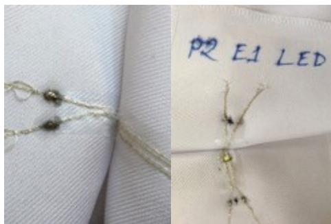
Figure 36. E1 bonding after wash/dry cycles.
