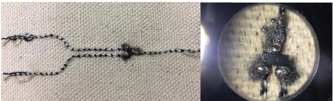
Figure 60: Stitched surface-mount sensor circuit: Stitched circuit (left) and microscopic view (right)
