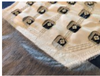
Figure 52: Laser cut holes exposing the underside of daisy-chained LEDs for ease of troubleshooting
