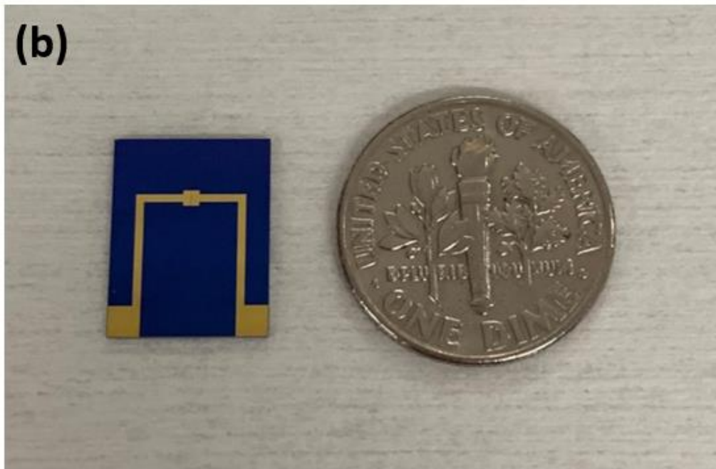
Figure 1.1 (a) Schematic of the graphene based IS-FET (b) Images of the fabricated sensor.
