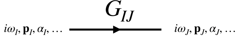
Figure 2.1: Diagrammatic representation of the Green's function, also called a propagator or two-point correlation function.
