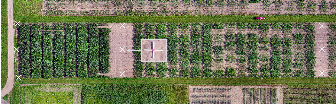
Figure 3.9. Ground control point placement throughout field border and internal alleys
