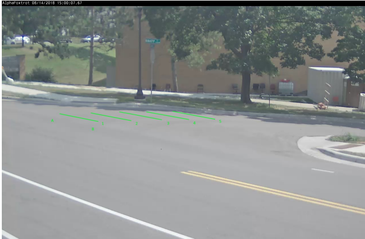
Figure 3.25 Camera view of the intersection of Como Ave and Knapp St with 5-ft overlay lines marked
