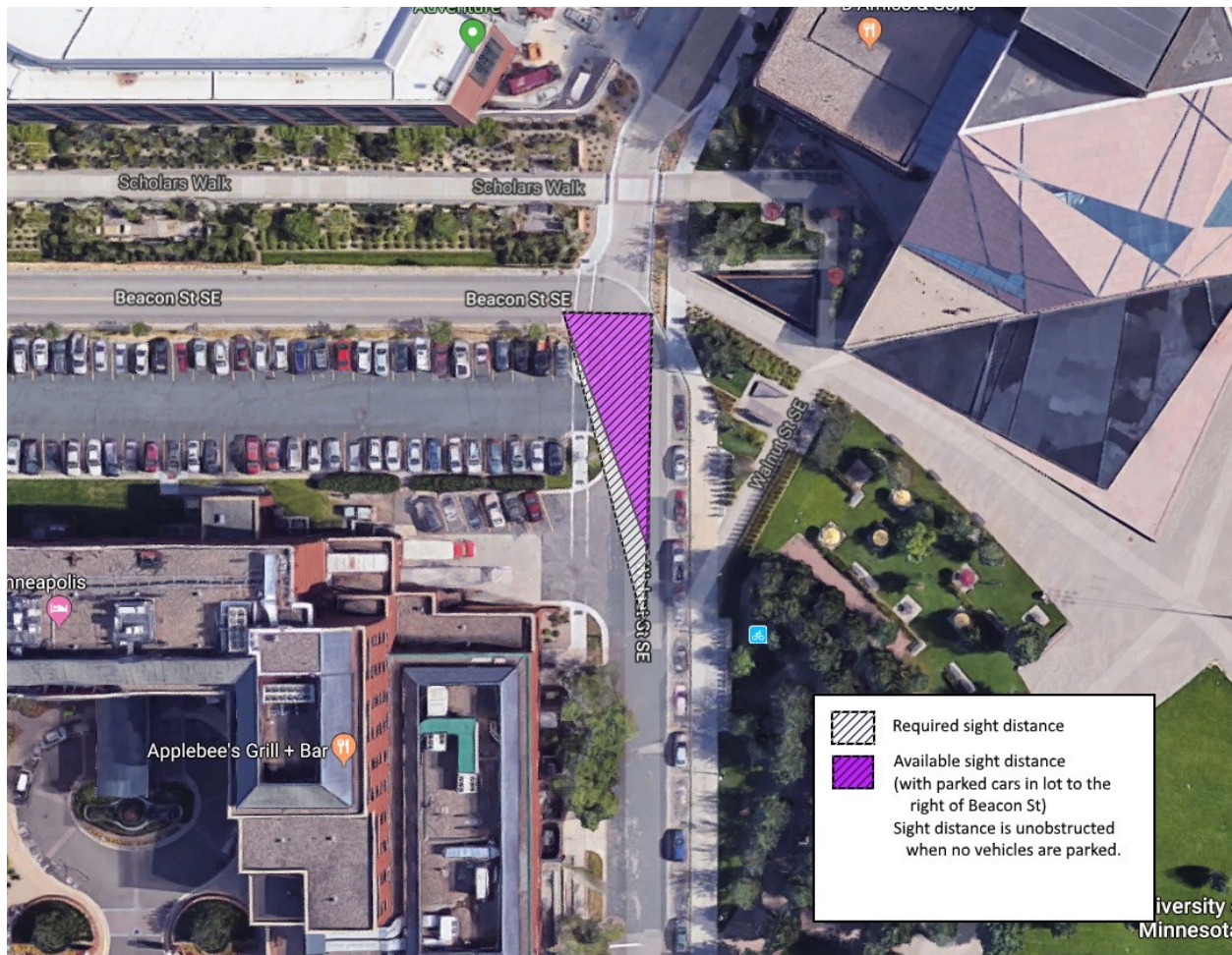
Figure 3.12 Available sight distance and required sight distance at Beacon St SE and Walnut St SE
