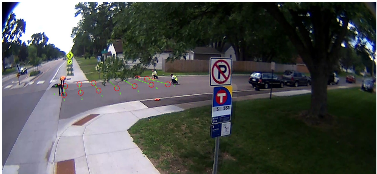
Figure 3.5 Calibration image for Site 190A with beads outlined in red (zoomed in)
