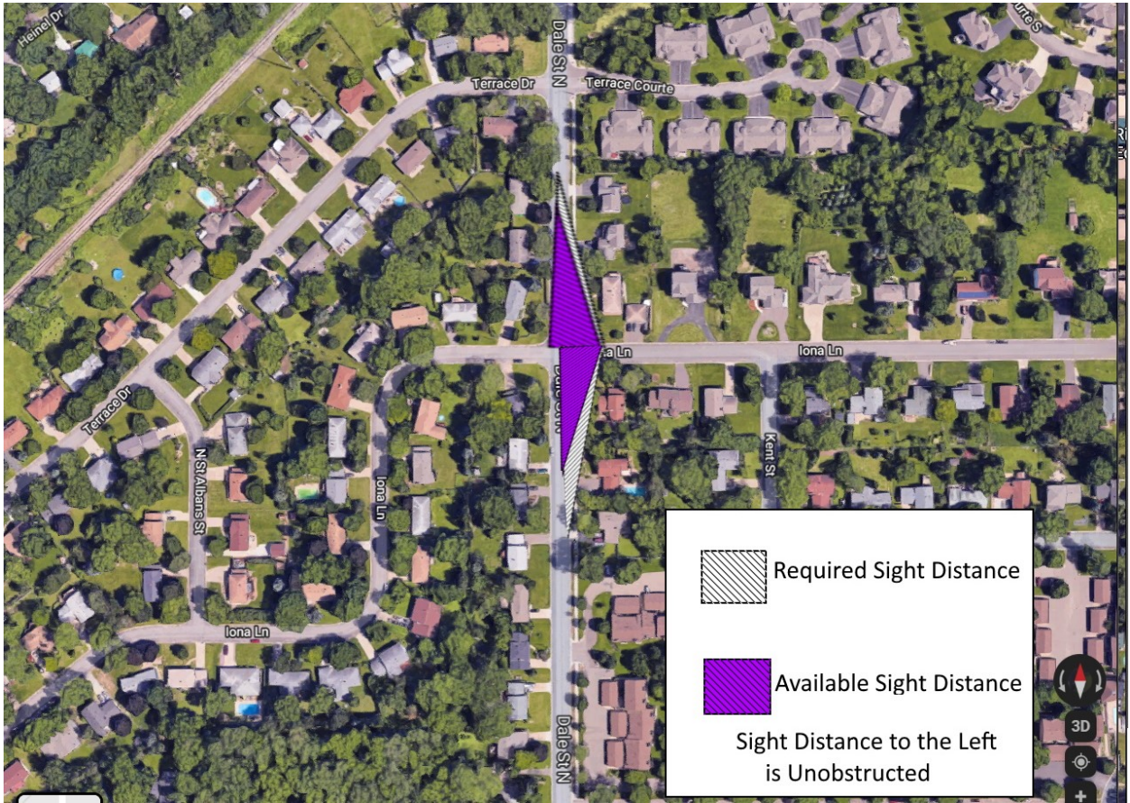
Figure 3.40 Available sight distance and required sight distance at Dale St N and Iona Ln
