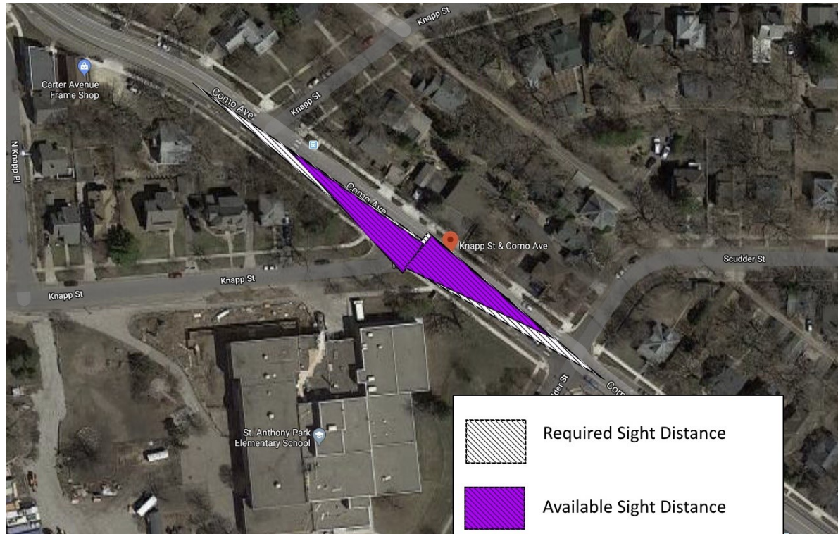
Figure 3.26 Available sight distance and required sight distance at Como Ave and Knapp St
