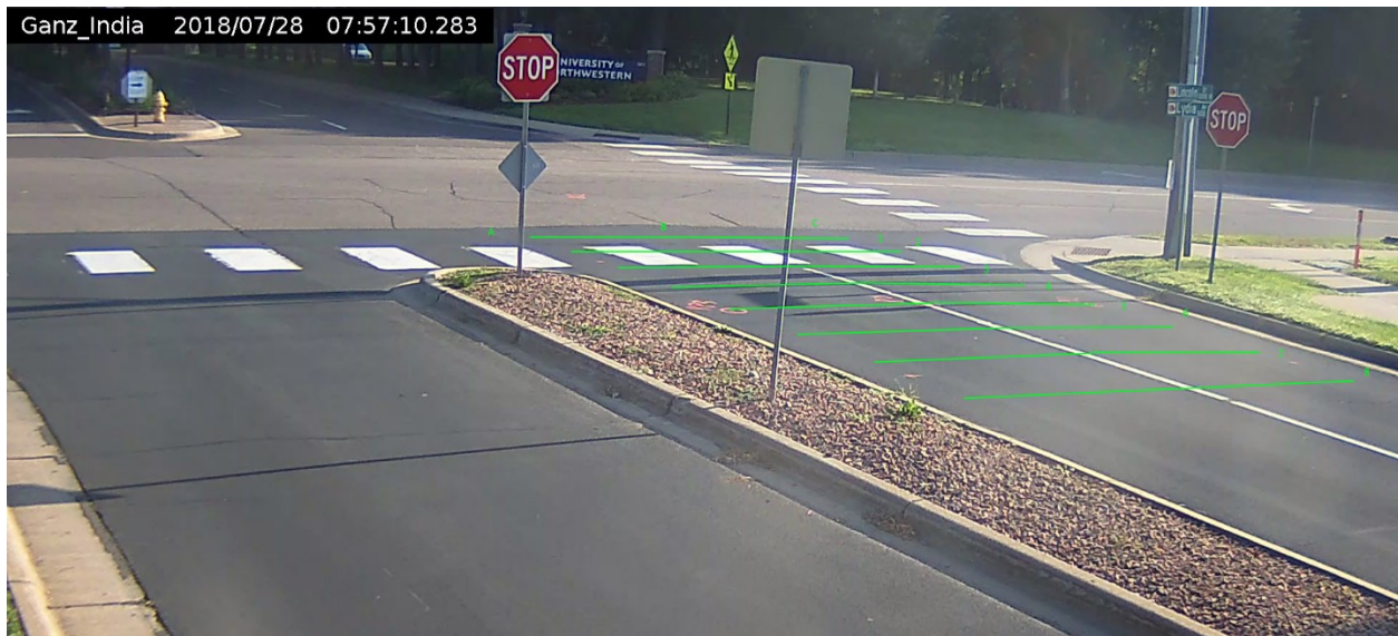
Figure 3.46 Camera view of the intersection of Lincoln Dr and Lydia Ave W with 5-ft overlay lines marked
