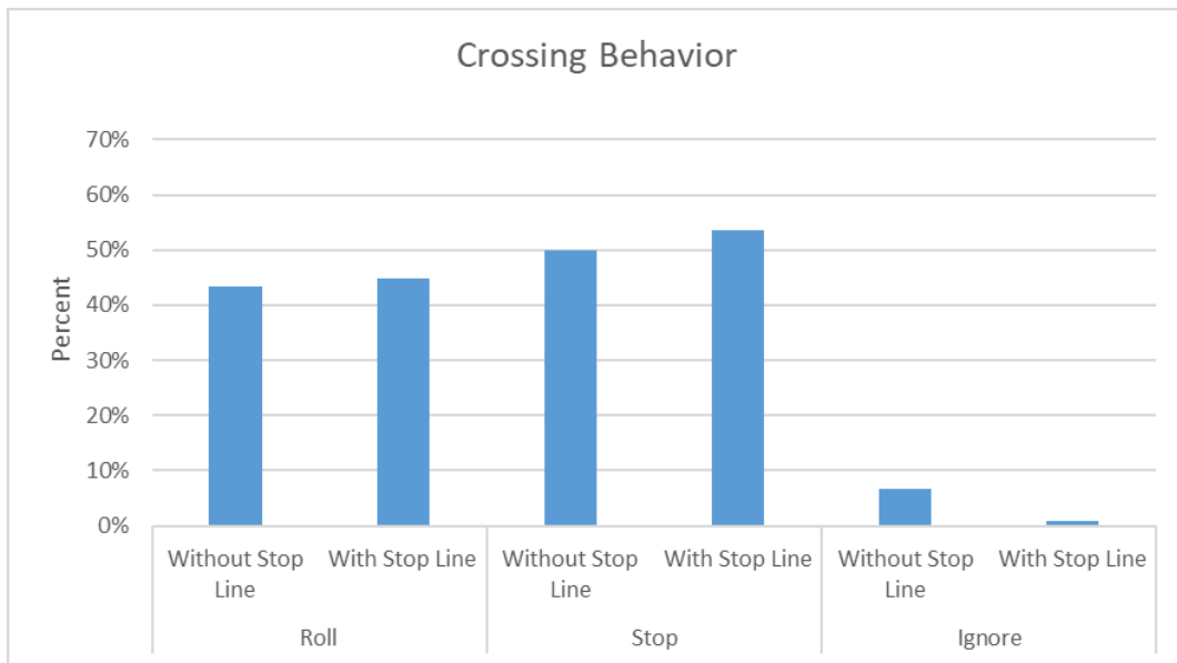
Figure 3.71 Portland Ave and 73rd St EB distribution of driver crossing behavior as a percentage of all events without- vs with-stop line
