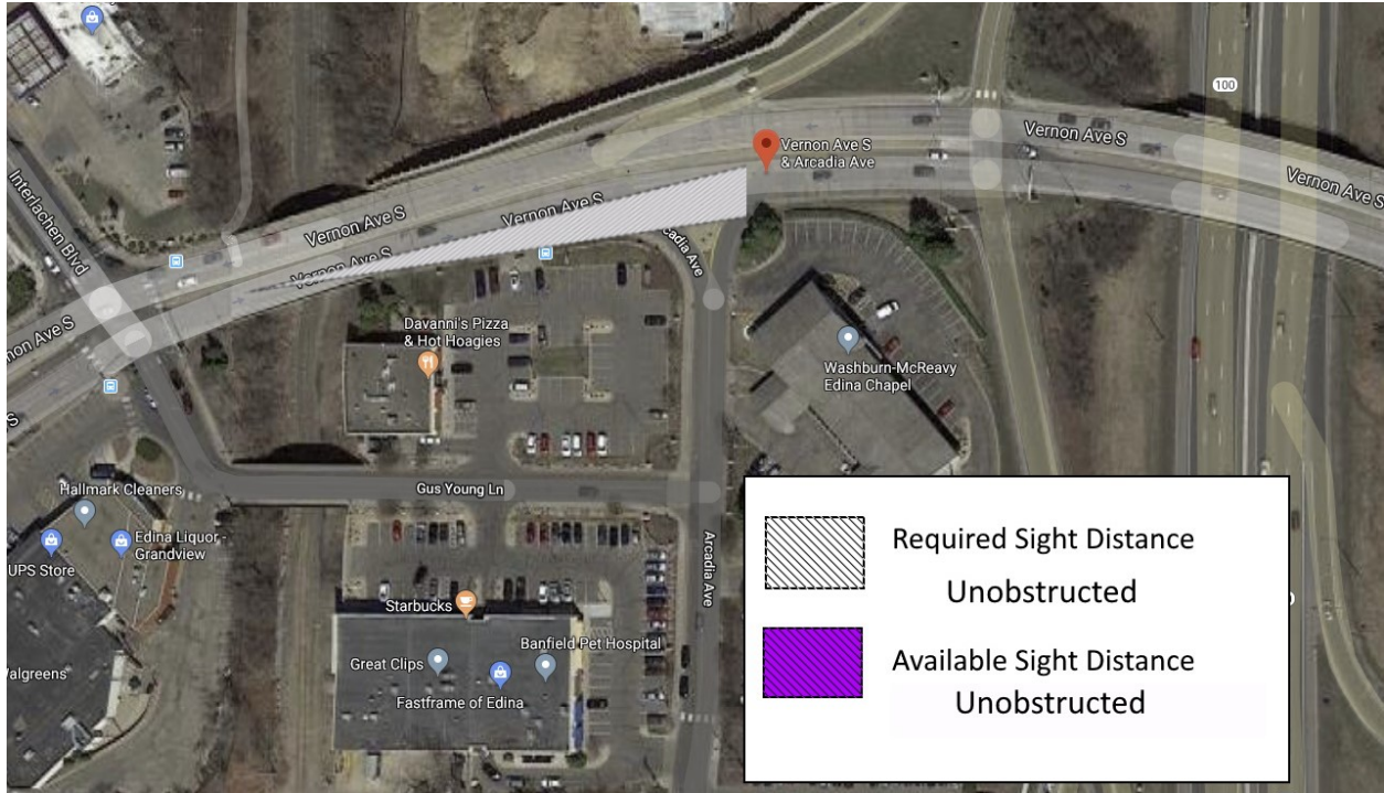
Figure 3.64 Available sight distance and required sight distance at Vernon Ave S and Arcadia Ave
