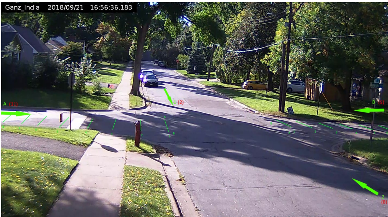
Figure 3.7 Raleigh Ave and W 28th St with-stop line reference image approach labels and reference lines (5-ft spacing)
