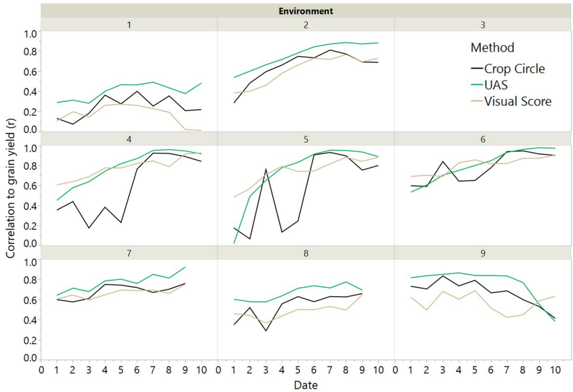
Figure 3-3. Pearson correlations between data collected approximately weekly and grain yield. Data was collected with an unmanned aircraft system (UAS) for passively sensed normalized difference vegetation index (NDVI), Crop Circle for ground based actively sensed NDVI, and by visual scores taken on a 1-5 scale.
