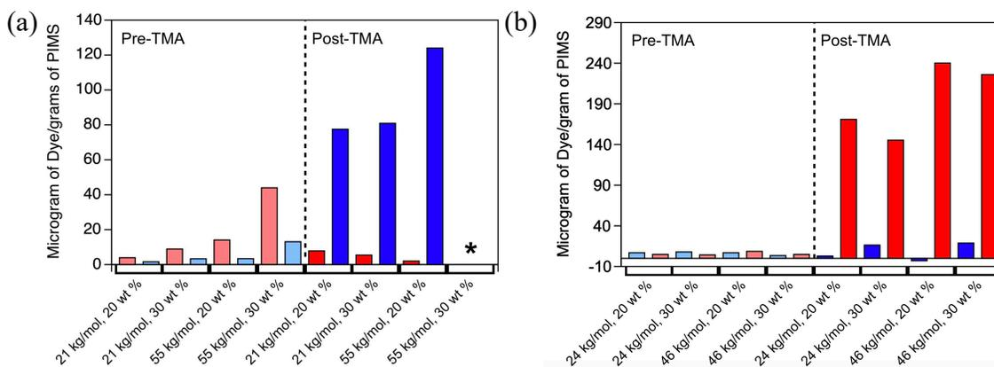
**Figure 3.7.** Dye absorption of methyl red (red) and toluidine blue (blue) dyes before and after TMA exposure for (a) PoSSE and (b) PVBC PIMS. \*PoSSE-55k-30 disintegrated during testing which increased solution turbidity enough to obscure UV absorption.
