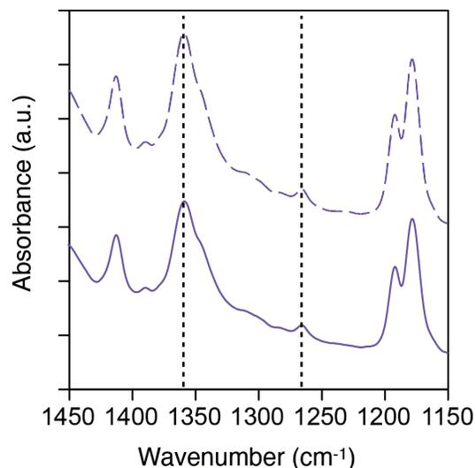
**Figure 2.25.** ATR-IR spectrum of PSSE<sub>260</sub>-P4ClS<sub>565</sub>-PVBC<sub>140</sub> triblock polymer before (solid plot) and after (dashed plot) exposure to 45% wt/wt trimethylamine vapor for 12 h. Vertical dashed lines are added as guides for the eye to note the C–Cl wag at 1266 cm<sup>-1</sup> and the S=O stretch at 1357 cm<sup>-1</sup>.
