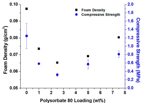
**Figure 5.6.** Density and compressive strength of 50 kg/mol 4-arm star PLA foamed at 23 °C with varying loadings of polysorbate 80.
