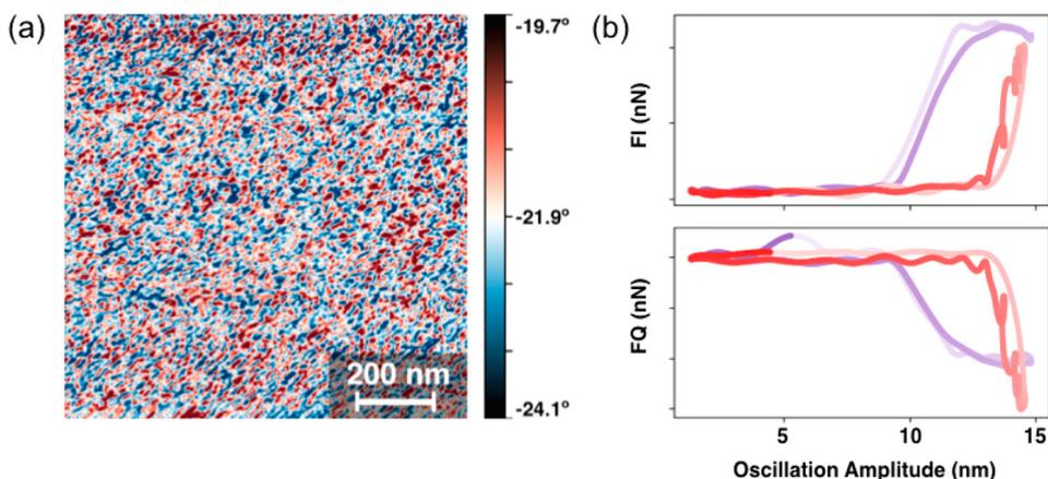
**Figure 2.28.** (a) Intermodulation AFM phase image of 57 nm thick film of PSSE<sub>110</sub>-P4CIS<sub>305</sub>-PVBC<sub>70</sub> triblock polymer after plasma etch and subsequent exposure to TMA vapor for 24 h. (b) Force (top) and dissipation (bottom) curves taken from a representative point within the blue domain (PSS, purple line) and red domain (PVBC, red line).
