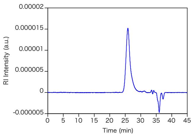
**Figure 2.3.** THF SEC chromatogram of  $\text{PS}_{140}\text{-}b\text{-PVBC}_{140}$
