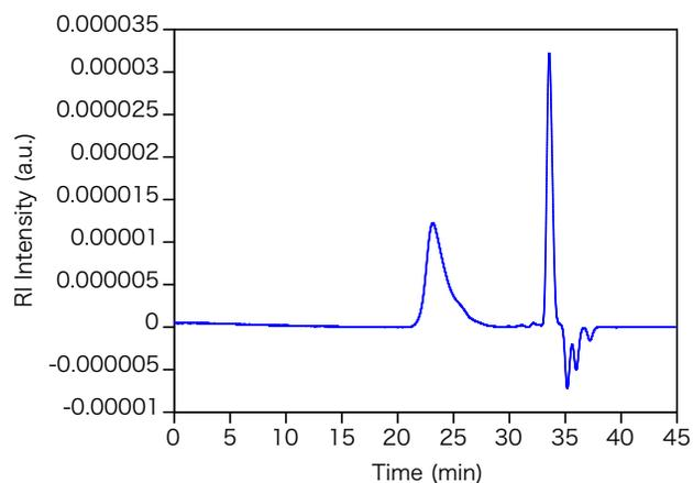
**Figure 2.12.** P4CIS<sub>700</sub>-PVBC<sub>110</sub> SEC Chromatogram
