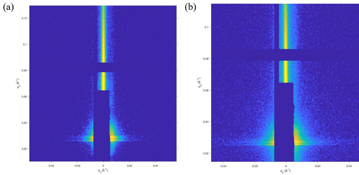
**Figure 2.8.** GISAXS scattering pattern of (a) PS<sub>710</sub>-PVBC<sub>400</sub> and (b) PS<sub>1290</sub>-PVBC<sub>650</sub> films after solvent vapor annealing in chlorobenzene. Incident angle of  $0.14^\circ$  and an exposure time of 20 s.
