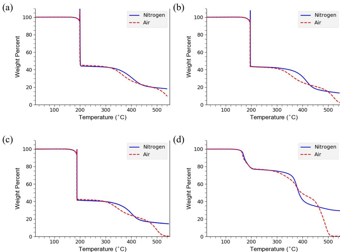
**Figure 4.9.** TGA analysis of PVBNO<sub>3</sub> under nitrogen (solid blue line) and air (dashed red line) with heating rates of (a) 20 °C min<sup>-1</sup>, (b) 10 °C min<sup>-1</sup>, (c) 5 °C min<sup>-1</sup>, and (d) 1 °C min<sup>-1</sup>
