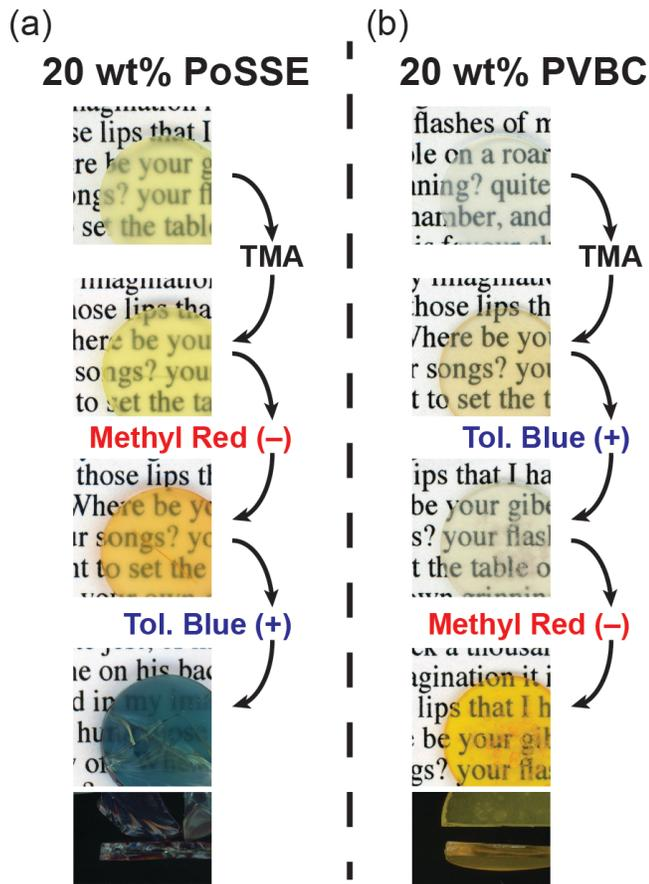
**Figure 3.4.** Images of (a) PoSSE-21k-20 and (b) PVBC-24k-20 monoliths as made, after functionalization with TMA, and after exposure to positively and negatively charged dyes.
