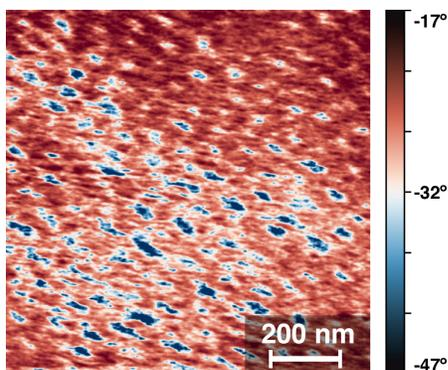
**Figure 4.14.** Intermodulation AFM image (see 2.3.12 ) of PS-*b*-PVBNO<sub>3</sub> diblock polymer spin coated on native silicon oxide wafer and solvent vapor annealed with chlorobenzene.
