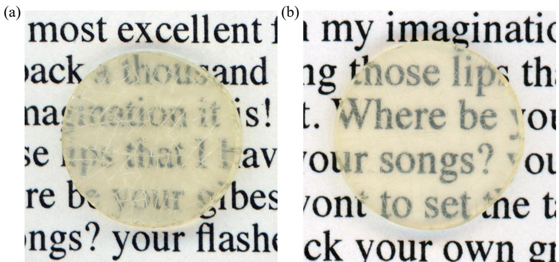
**Figure A.9.** Images of PVBC reverse PIMS with (a) PS and (b) P4CIS macroinitiators after soaking in TMA.
