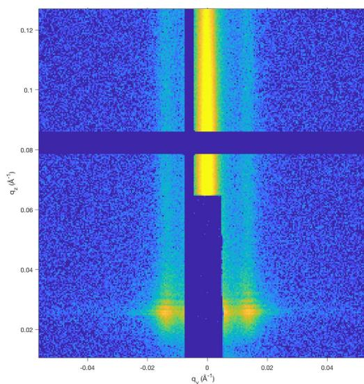
**Figure 2.19.** GISAXS scattering pattern of PSSE<sub>260</sub>-P4ClS<sub>1585</sub> film after solvent vapor annealing in chlorobenzene. Incident angle of 0.14° and an exposure time of 20 s.
