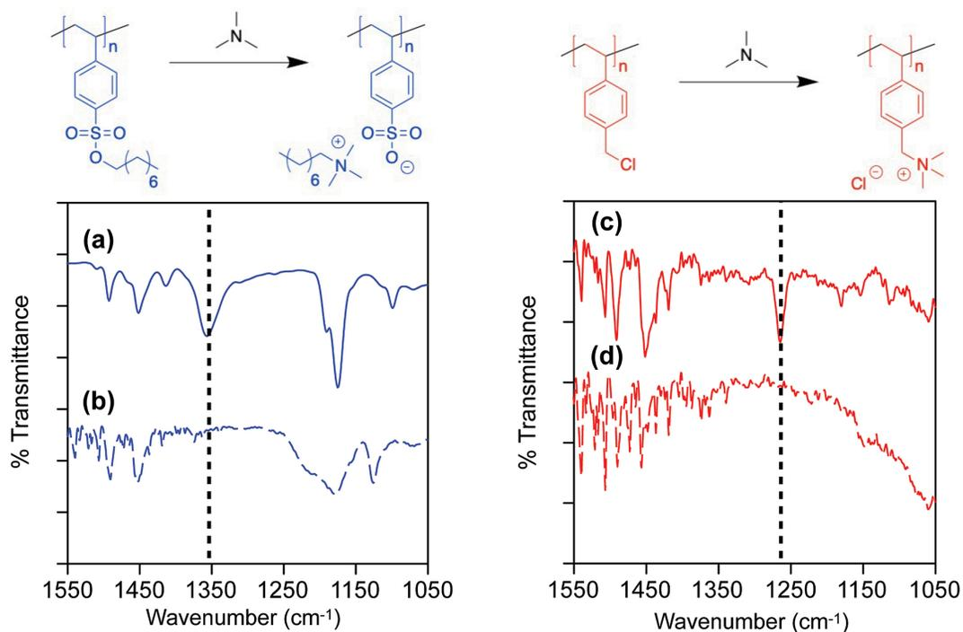
**Figure 3.6.** ATR-IR of (a) unfunctionalized and (b) TMA exposed PoSSE-62k-30 PIMS and (c) unfunctionalized and (d) TMA exposed PVBC-24k-20 PIMS.
