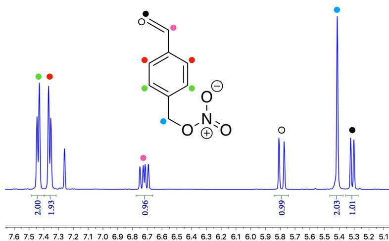
**Figure 4.1.** <sup>1</sup>H NMR spectrum of VBNO<sub>3</sub>
