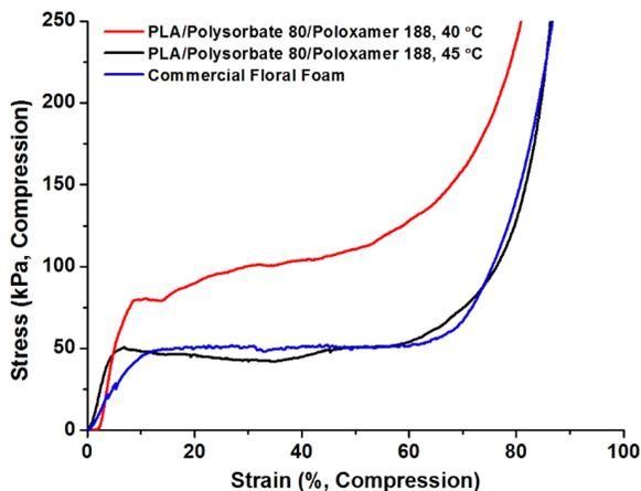
**Figure 5.10.** Compression stress versus strain curves for a commercial phenolic-based floral foam and PLA foams prepared with a 90:5:5 wt% 4-arm PLA:polysorbate 80:poloxamer 188 formulation foamed at 40 and 45 °C.
