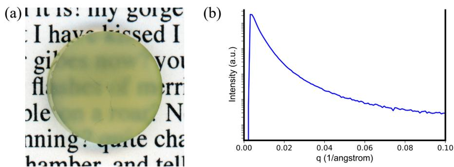
**Figure A.5.** (a) Image and (b) SAXS spectrum for (62k PoSSE)-(146k P4ClS)-(61k PVBC) PIMS.
