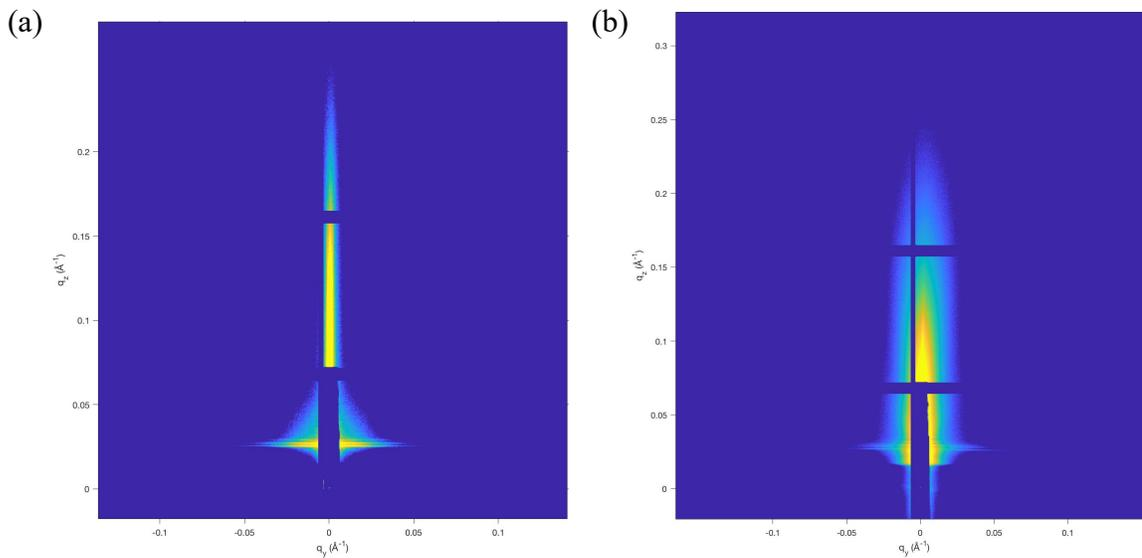
**Figure 2.6.** GISAXS scattering pattern of PS<sub>140</sub>-PVBC<sub>140</sub> film after solvent vapor annealing in chlorobenzene (a) before and (b) after exposing to TMA vapor for 1 hour. Incident angle of 0.14° and an exposure time of 20 s.
