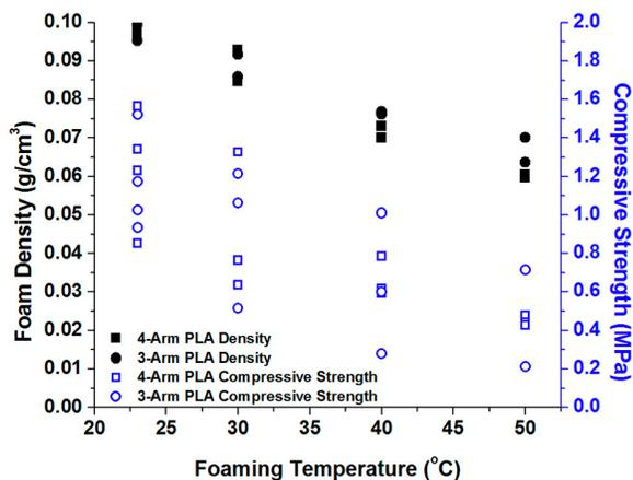
**Figure 5.4.** Plot of compressive strength versus foaming temperature for PLA foams prepared with 3-arm and 4-arm PLA of comparable molar mass (ca. 50 kg/mol).
