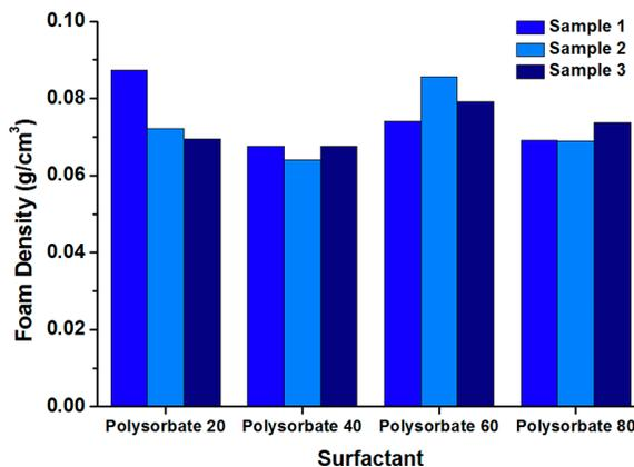
**Figure 5.5.** Density of foams prepared with a variety of polysorbate surfactants at 22 °C with 95:5 wt:wt loading of 50 kg/mol 4-arm PLA:polysorbate. Results of density determination for three samples of each polysorbate composition are presented.
