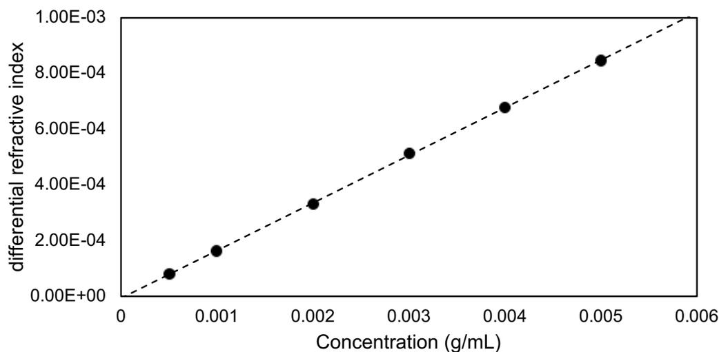
**Figure 3.1.** Batch  $dn/dc$  measurement for poly(vinylbenzyl chloride). Final  $dn/dc = 0.1710 \pm 0.0007 \text{ mL g}^{-1}$ .
