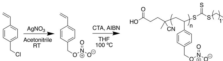
**Scheme 4.1.** Synthetic scheme for the synthesis of VBNO<sub>3</sub> and PVBNO<sub>3</sub>.
