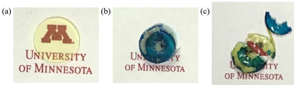
**Figure A.1.** PoSSE/PVBC blend PIMS (a) as made, (b) after exposure to TMA and toluidine blue solution, and (c) after exposure to methyl red.
