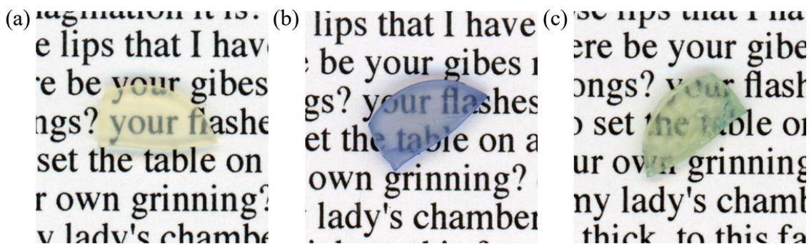
**Figure A.7.** PIMS monolith containing 30 wt% PoSSE–P4CIS–PVBC triblock polymer (a) after TMA exposure, (b) after exposure to toluidine blue solution, and (c) after exposure to methyl red solution.
