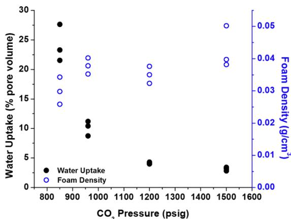
**Figure 5.9.** Plot of water uptake and density versus CO<sub>2</sub> treatment pressure for 90:5:5 wt% PLA:polysorbate 80:poloxamer 188 foamed at 55 °C.
