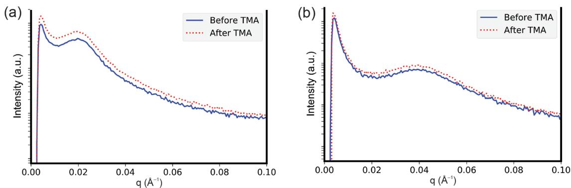
**Figure 3.5.** Transmission SAXS data of (a) a representative PoSSE-55k-20 PIMS (solid blue line) before and (dotted red line) after TMA exposure and (b) PVBC-24k-20 (solid blue line) before and (dashed red line) after TMA exposure.
