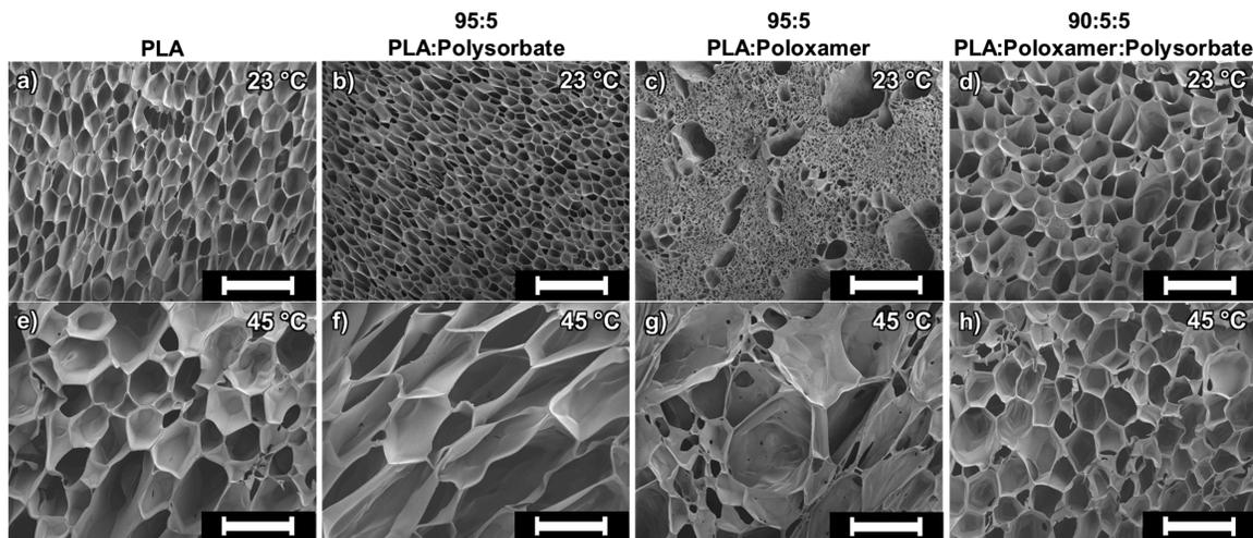
**Figure 5.11.** Scanning electron microscope images of PLA and PLA/surfactant blend foams prepared at (a–d) 23 °C and (e–h) 45 °C. All foams were prepared with 4-arm PLA ( $M_n = 50.5$  kg/mol) and the surfactants were polysorbate 80 and poloxamer 188 incorporated at 5 wt% loadings. Scale bars are 1 mm.
