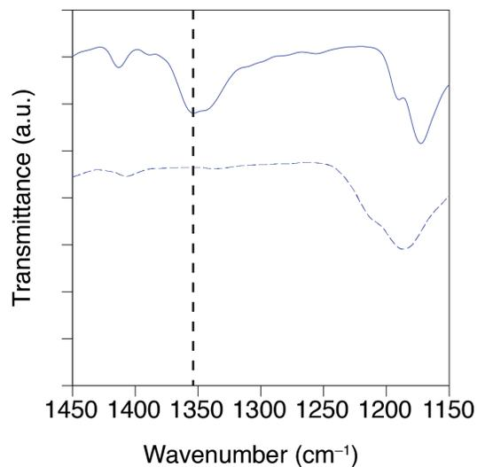
**Figure 2.20.** FT-IR spectrum of PSSE homopolymer before (solid line) and after (dashed line) exposure to 45% wt/wt trimethylamine solution for 8 h at 80 °C. Dashed lines are added as guides for the eye to note the S=O stretch at 1350 cm<sup>-1</sup>.
