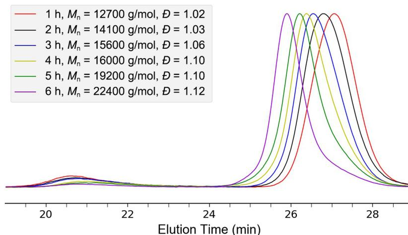
**Figure 4.8.** Normalized differential refractive index data of PVBNO<sub>3</sub> over a 6 hr polymerization.  $M_n$  and  $D$  were calculated using SEC. Corresponding  $M_n$  by NMR: 1 h = 20.3 kg · mol<sup>-1</sup>, 2 h = 25.3 kg · mol<sup>-1</sup>, 3 h = 31.4 kg · mol<sup>-1</sup>, 4 h\* = 50.8 kg · mol<sup>-1</sup>, 5 h\* = 70.1 kg · mol<sup>-1</sup>, 6 h\* = 56.3 kg · mol<sup>-1</sup>. \*indicates poor end group resolution by NMR.
