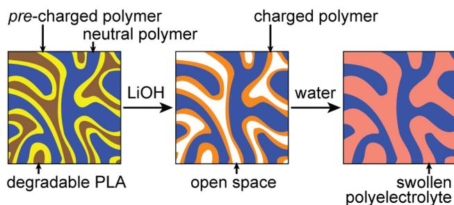
**Figure B.4.** Diagram of PIMS synthesized with a *pre*-charged domain and a degradable PLA domain which will etch out when functionalized, leaving open space for the polyelectrolyte to swell with water.
