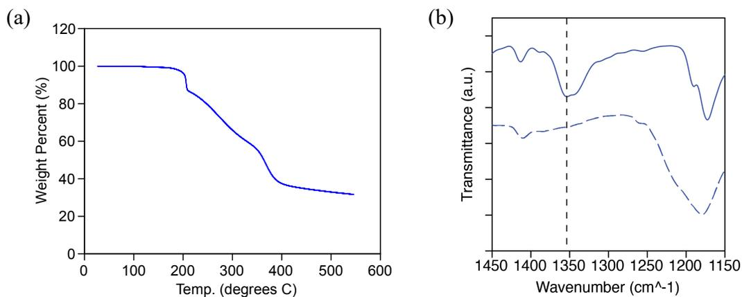
**Figure 2.16.** (a) TGA plot of PSSE. (b) FT-IR spectrum of PSSE homopolymer before (solid plot) and after (dashed plot) exposure to 30 wt. % NaOH in 5:6 vol./vol. of H<sub>2</sub>O/MeOH for 48 h at 70 °C. Dashed vertical line is added as a guide for the eye to note the S=O stretch at 1350 cm<sup>-1</sup>.
