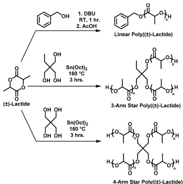
**Scheme 5.1.** Synthesis of Linear and Star-Shaped PLA via ROTEP.
