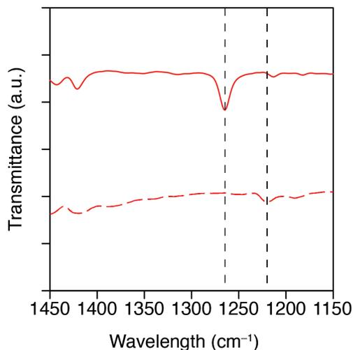
**Figure 2.4.** FT-IR spectrum of PVBC homopolymer before (solid line) and after (dashed line) exposure to 45% wt/wt trimethylamine solution for 17 h at 60 °C. Dashed lines are added as guides for the eye to note the C–Cl wag at 1266 cm<sup>-1</sup>, the C–N stretch at 1220 cm<sup>-1</sup>.
