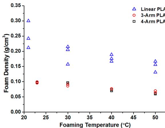
**Figure 5.3.** PLA foam density versus CO<sub>2</sub> foaming temperature for linear, 3-arm star, and 4-arm star PLA with comparable molar masses of 46, 51, and 51 kg/mol, respectively.
