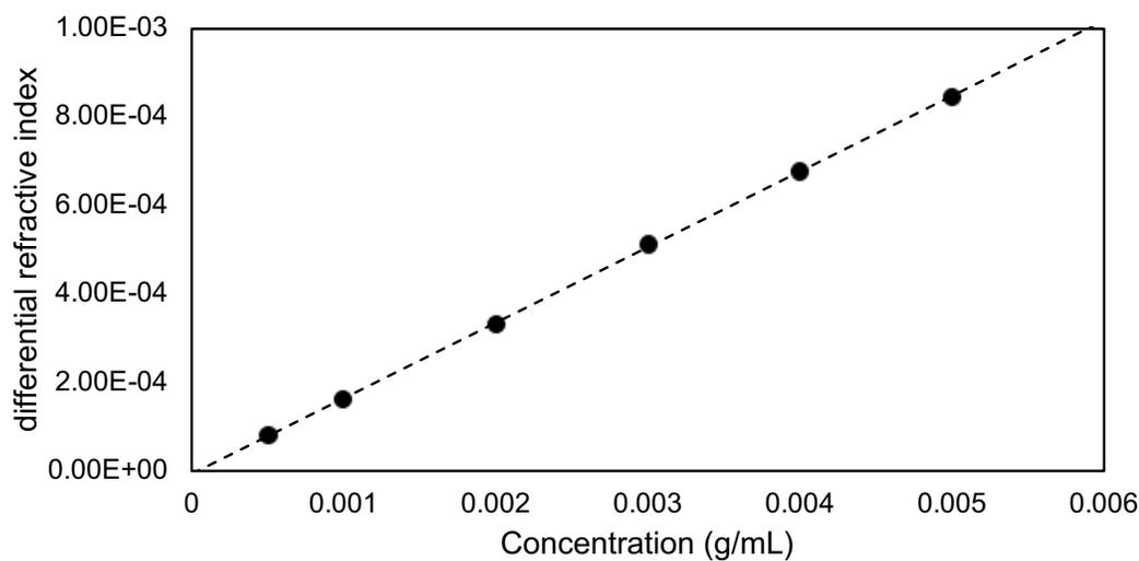
**Figure 3.2.** Batch  $dn/dc$  measurement for poly(vinylbenzyl chloride). Final  $dn/dc = 0.1156 \pm 0.0009 \text{ mL g}^{-1}$ .
