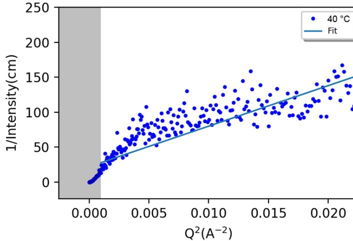
**Figure 4.6.** Representative  $I^{-1}(q)$  v.  $q^2$  plot for  $40 \text{ }^\circ\text{C}$ . The shaded region at low  $q$  represents data that is excluded from the linear fit.
