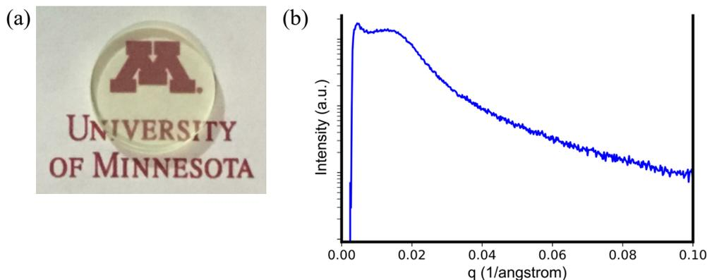
**Figure A.3.** (a) Image and (b) SAXS data for PoSSE-*b*-PVBC diblock PIMS.
