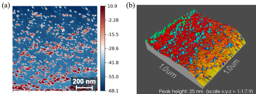
**Figure 2.27.** Intermodulation AFM scan of PSSE<sub>110</sub>-P4CIS<sub>305</sub>-PVBC<sub>70</sub> after plasma etching (a) the phase image scan and (b) the scanned image with the height data overlaid on the phase data.
