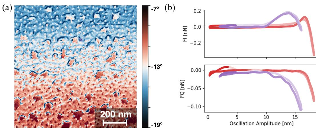
**Figure 2.13.** (a) An intermodulation AFM scan of P4CIS<sub>700</sub>-PVBC<sub>110</sub> after TMA exposure and (b) the force (top) and dissipation (bottom) curves where the red “X” and lines correspond to a PVBAC domain and the purple “X” and lines correspond to a P4CIS domain.
