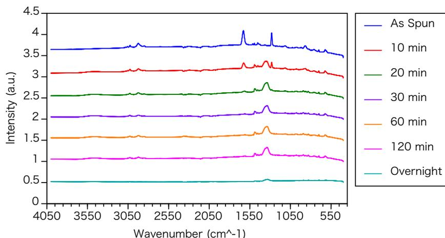
**Figure 4.12.** ATR-IR spectra of PS–PVBNO<sub>3</sub> films on silicon wafer substrates exposed to trimethylamine vapor for varying periods of time: as spun (blue), 10 min (red), 20 min (green), 30 min (purple), 60 min (orange), 120 min (magenta), and overnight (teal).
