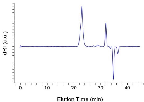
**Figure B.2.** SEC chromatogram of PLA synthesized with pentanol CTA.
