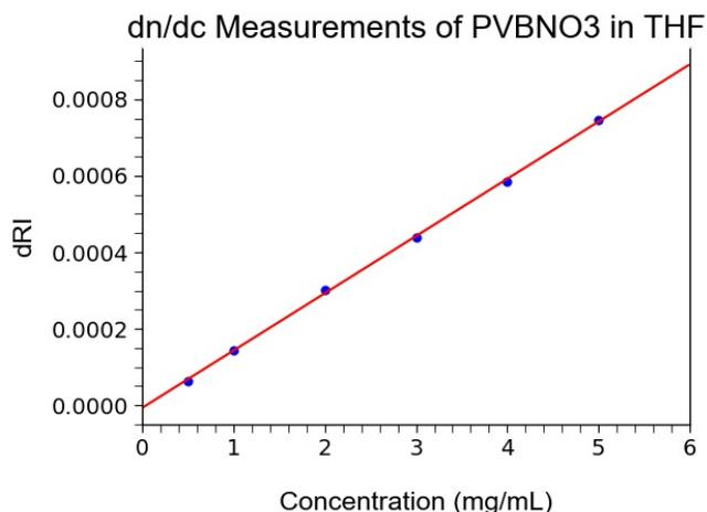
**Figure 4.4.**  $dn/dc$  measurement of PVBNO<sub>3</sub> in THF, giving a slope of  $0.1494 \pm 0.0018$  mL g<sup>-1</sup>.
