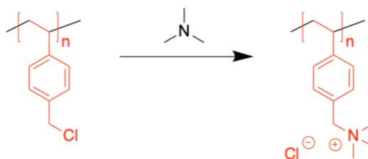
**Scheme 2.2.** Conversion of the Neutral Homopolymers to Their Ionic Counterparts: (A) Poly(*n*-propyl styrene sulfonic ester) (PSSE) is exposed to trimethylamine, and the propyl group undergoes an SN<sub>2</sub> reaction to form poly(styrene sulfonate) (PSS). (B) Poly(vinylbenzyl chloride) (PVBC) is exposed to trimethylamine, and the benzyl chloride
