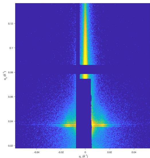
**Figure 2.24.** GISAXS scattering pattern of PSSE<sub>110</sub>-P4ClS<sub>305</sub>-PVBC<sub>70</sub> film after solvent vapor annealing in chlorobenzene. Incident angle of 0.14° and an exposure time of 20 s.
