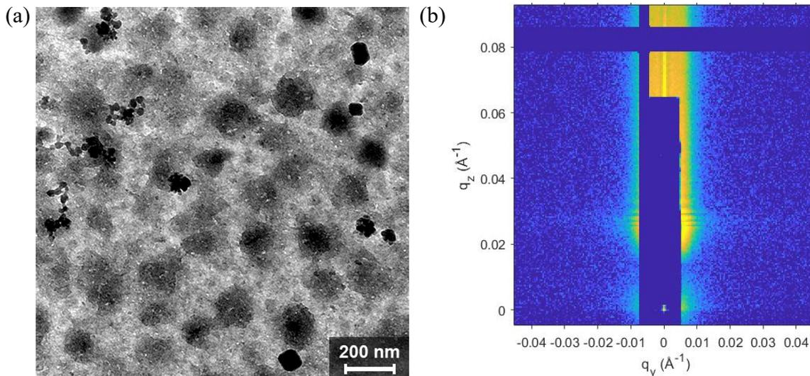
**Figure 2.14.** (a) Transmission electron microscopy image of P4ClS<sub>700</sub>-PVBC<sub>110</sub> 50 nm thick film after solvent vapor annealing with chlorobenzene and staining by submersion in a 0.1 wt% aqueous solution of phosphotungstic acid. (b) GISAXS scattering pattern of P4ClS<sub>700</sub>-PVBC<sub>110</sub> film after solvent vapor annealing in chlorobenzene. Incident angle of 0.14° and an exposure time of 20 s.
