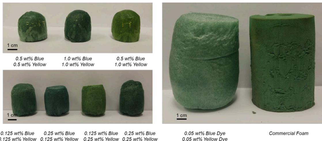
**Figure 5.13.** Photographs of foams with colorant additives composed of the 90:5:5 4-arm PLA:polysorbate 80:poloxamer 188 formulation and Keyplast™ dyes incorporated at the indicated loading as an additive wt% relative to the total mass of the PLA and surfactant blend. All samples were foamed at 50 °C with 6 MPa (gauge pressure CO<sub>2</sub>). A commercial phenolic floral foam is shown for comparison.
