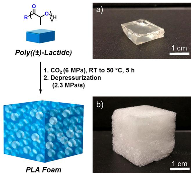
**Figure 5.2.** Schematic of PLA foaming using CO<sub>2</sub> as a physical blowing agent with representative images of PLA (a) before and (b) after CO<sub>2</sub> treatment and subsequent rapid depressurization.
