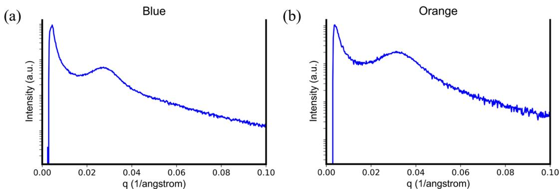
**Figure A.2.** Transmission SAXS data for (a) blue and (b) orange portions of the PoSSE/PVBC blend PIMS.
