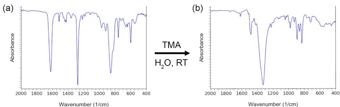
**Figure 4.11.** ATR-IR of (a) PVBNO<sub>3</sub> and (b) PVBAN showing the disappearance of nitrate ester peaks at 1275 cm<sup>-1</sup> and 1622 cm<sup>-1</sup> and appearance of ammonium peaks at 1326 cm<sup>-1</sup> and 1480 cm<sup>-1</sup>.
