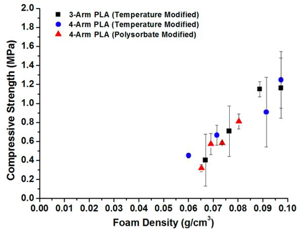
**Figure 5.7.** Plot of compressive strength versus density for PLA based foams with density modified by foaming at temperatures from 22 to 50 °C (3-arm PLA and 4-arm PLA) and polysorbate 80 incorporation at loadings of 1, 2.5, 5, and 7.5 wt%.
