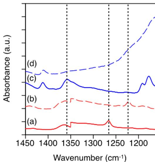
**Figure 2.15.** ATR-IR spectra of 1  $\mu\text{m}$  thick films of diblock polymers P4ClS<sub>700</sub>-PVBC<sub>110</sub> (a) before and (b) after 1 h of TMA exposure and PSSE<sub>260</sub>-P4ClS<sub>1585</sub> (c) before and (d) after 12 h of TMA exposure. Black dashed lines are added to highlight the C-Cl wag at 1266  $\text{cm}^{-1}$ , the C-N stretch at 1220  $\text{cm}^{-1}$ , and the S=O stretch at 1357  $\text{cm}^{-1}$ .
