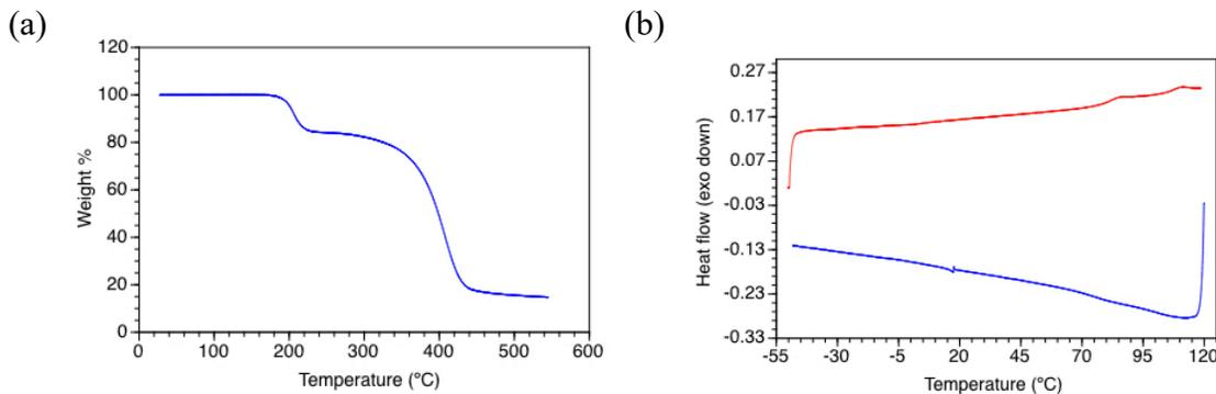
**Figure 4.13.** (a) TGA analysis of PS–PVBNO<sub>3</sub> under nitrogen with a heating rate of 10 °C min<sup>-1</sup> and (b) DSC analysis of PS–PVBNO<sub>3</sub> (10 °C min<sup>-1</sup> heating rate, 2nd heating curve shown)
