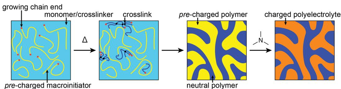
**Figure 3.3.** Schematic of polymerization-induced microphase separation to create percolating charged domains.
