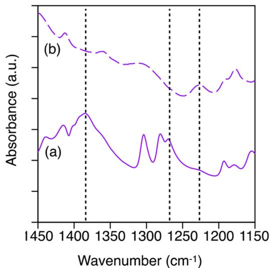
**Figure 2.26.** ATR-IR spectra of 57 nm thick films of plasma-etched triblock polymers PSSE<sub>110</sub>–P4CIS<sub>305</sub>–PVBC<sub>70</sub> (a) before (solid) and (b) after (dashed) exposure to TMA. Black dashed lines are added as guides for the eye to note the C–Cl wag at 1266 cm<sup>-1</sup>, the C–N stretch at 1220 cm<sup>-1</sup>, and the S=O stretch at 1357 cm<sup>-1</sup>.
