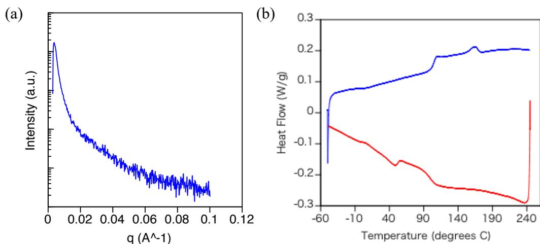
**Figure 2.10.** (a) Transmission SAXS 1D plot and (b) DSC plot of PS<sub>140</sub>-PVBC<sub>140</sub>.
