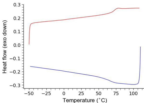
**Figure 4.10.** DSC analysis of PVBNO<sub>3</sub> (10 °C min<sup>-1</sup> heating rate, 2nd heating curve shown)
