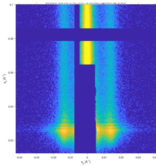
**Figure 2.21.** GISAXS scattering pattern of PSSE<sub>260</sub>-P4ClS<sub>1585</sub> film after solvent vapor annealing in chlorobenzene and exposure to 45% wt/wt trimethylamine solution vapors. Incident angle of 0.14° and an exposure time of 20 s.
