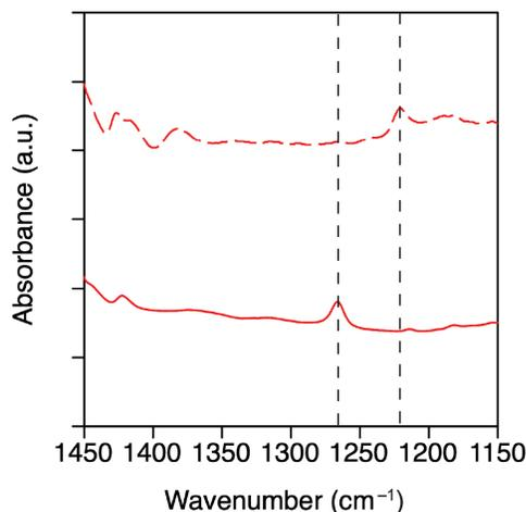
**Figure 2.5.** ATR-IR spectrum of PS<sub>140</sub>-PVBC<sub>140</sub> before (solid line) and after (dashed line) exposure to 45% wt/wt trimethylamine vapor for 1 h. Dashed lines are added as guides for the eye to note the C–Cl wag at 1266 cm<sup>-1</sup>, the C–N stretch at 1220 cm<sup>-1</sup>.
