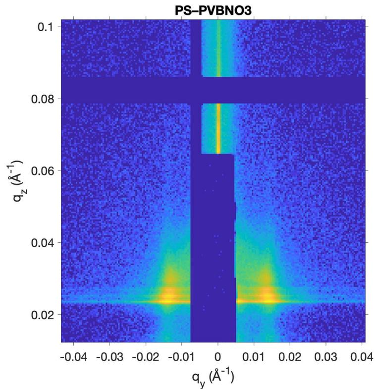
**Figure 4.15.** GISAXS of 87 nm thick film of (134k PS)-*b*-(37k PVBNO<sub>3</sub>) on native silicon oxide showing vertical features scattering at  $q_y = 0.015 \text{ \AA}^{-1}$ .
