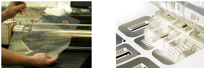
Figure 1.1: Electronic circuits printed on flexible substrates [1, 2].
