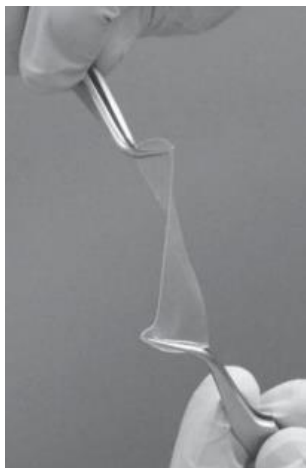
Figure 1.2: Image of free-standing ion gel of 20% copolymer of vinylidene fluoride and hexafluoropropylene P(VDF-HFP) in [EMIM][TFSI]. Reproduced with permission from ref. 52. Copyright 2012 Wiley.
