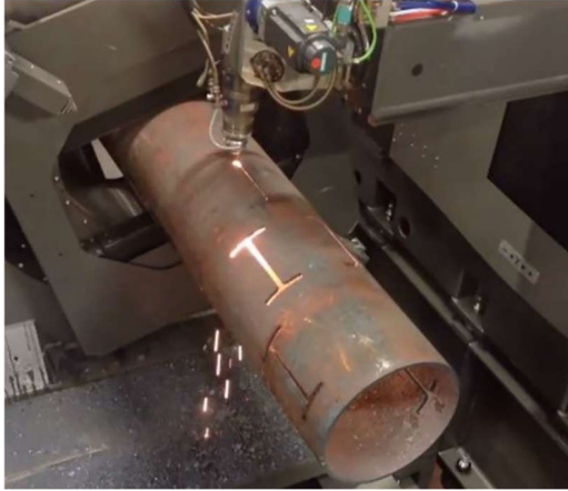
(a) Laser cutting process on a tubular profile
