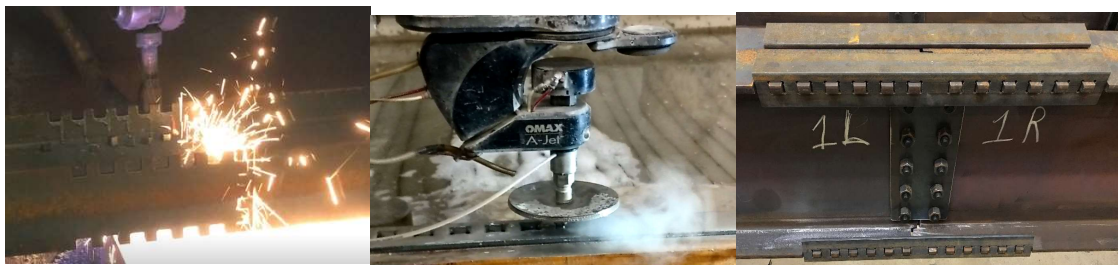
(a) Cutting process (b) Final product Fig. 3-4: Manufacturing the intermeshed connection
