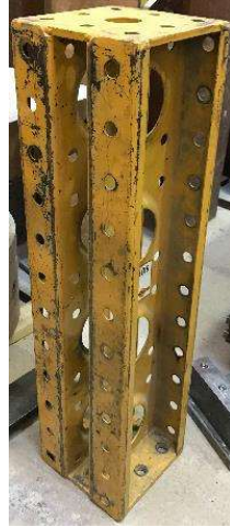
(a) EFCO members for Test 1 and Test 2
