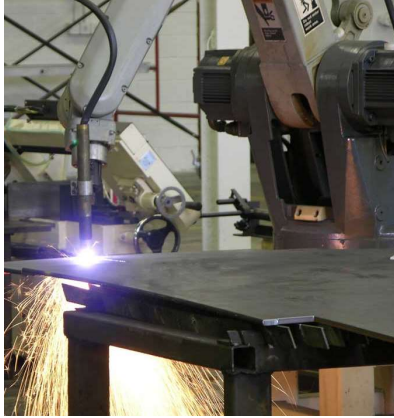
(a) Plasma cutting performed by an industrial robot [3]
