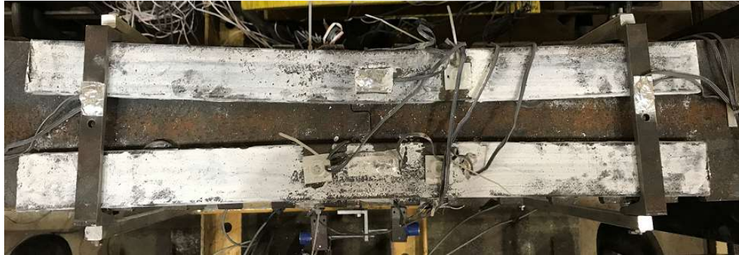
(a) Kinking of compression angle due to lateral-torsional buckling of the specimen
