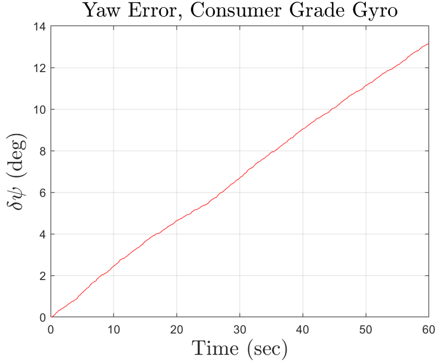
Figure 2.15 Yaw error propagation with noisy gyro.
