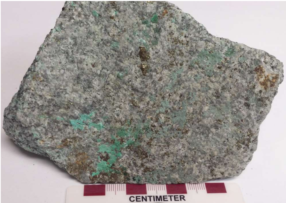
Figure 5.4 Hand sample of Bag-1, a quartz monzonite that contains very fine-grained disseminated chalcopyrite.
