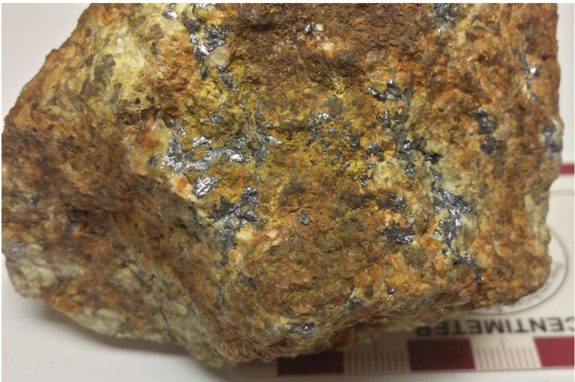
Figure 5.6 Hand sample of O-219, an iron stained quartz monzonite with silver-grey molybdenite smeared on the surface. The texture of the ore in this sample appears as interconnected clots.
