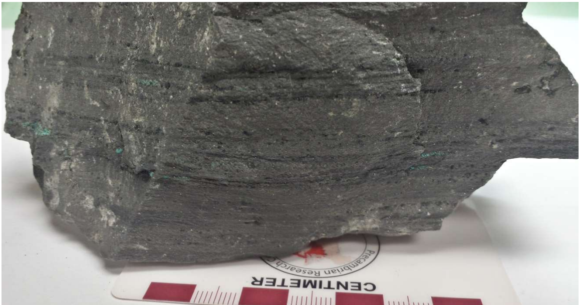
Figure 5.10 Hand sample of 1716, Nonesuch Shale with chalcocite and native copper, represented by greenish-blue and black oxidation, occurring in a stratiform pattern.
