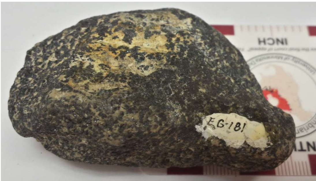
Figure 5.1 Hand sample of EG-181. The black submetallic mineral is chromite, which dominates the sample with weathered dunite filling in the matrix. The chromite exhibits cumulate texture with intercumulate olivine.
