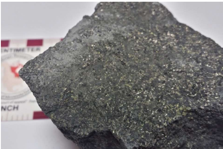
Figure 5.2 Hand sample of Eagle-1. The black gangue material is peridotite while the yellowish metallic portion is a mixture of chalcopyrite, pentlandite, and pyrrhotite which are all occurring as a disseminated texture.
