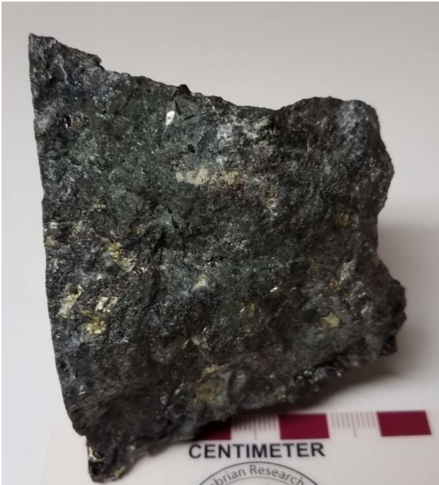
Figure 5.3 Hand sample of DC, a gabbroic rock that contains sulfide blebs of both chalcopyrite and pentlandite. The ore minerals here have a clotted texture or a mix of both fine- and coarse-grained disseminated ore.
