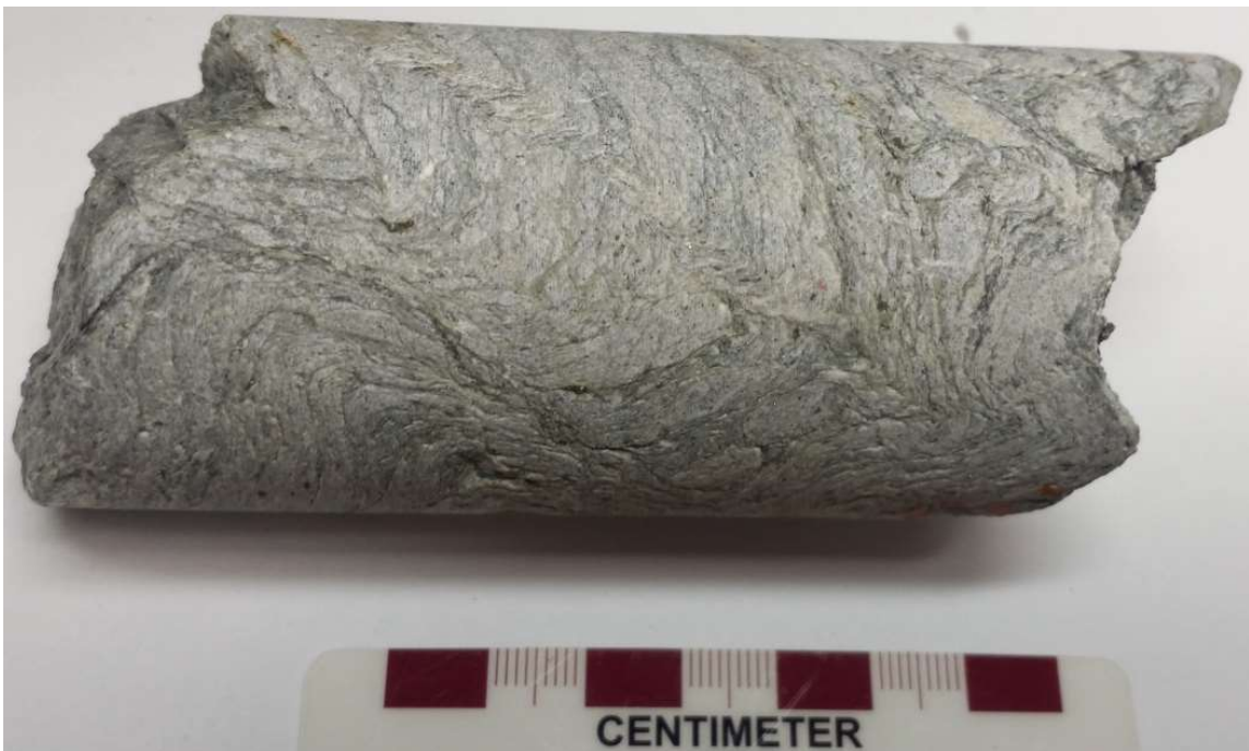
Figure 5.5 Hand sample of V-1, a highly altered portion of a porphyry deposit. Show here is highly altered gangue material, mostly sericite, quartz, with minor chlorite. Not pictured because of the small size are both chalcopyrite and pyrite which are sparsely disseminated throughout.
