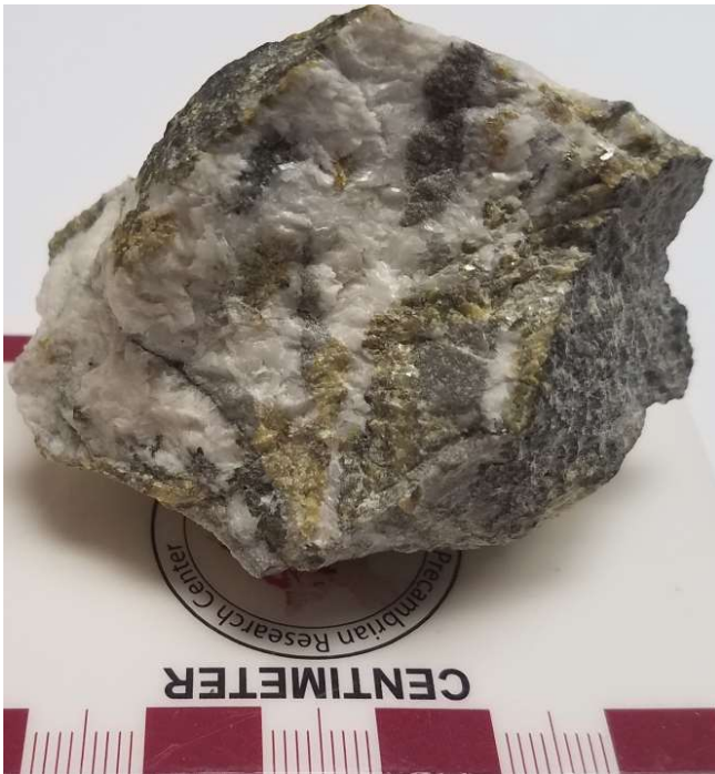
Figure 5.9 Hand sample of MVT-1, a brecciated limestone (dark grey) that has had sphalerite (light yellow), chalcopyrite (not pictured), and calcite (milky white) fill in the void space.
