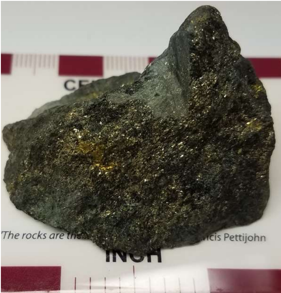
Figure 5.8 Hand sample of SLC-2476, chlorite stringer containing fine-grained pyrite and chalcopyrite.
