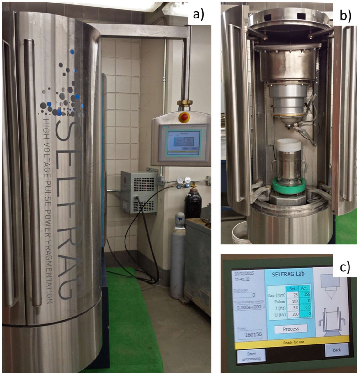
Figure 4.1 SELFRAG High Voltage Power Fragmentation EPD device with the sample chamber doors closed and touch panel controls (a). Sample chamber doors open displaying the sample vessel resting on the green lifting platform (b). Close-up of the control panel displaying the 4 variables that can be adjusted before sample processing (c); see 4.2.2 for details.
