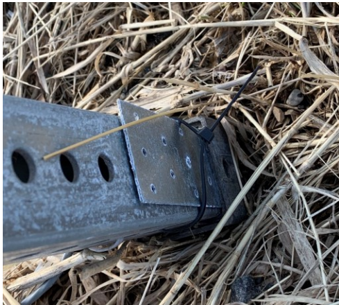
Figure 8.28 - RICWS breakaway slip-base post connection with shim inserted.
