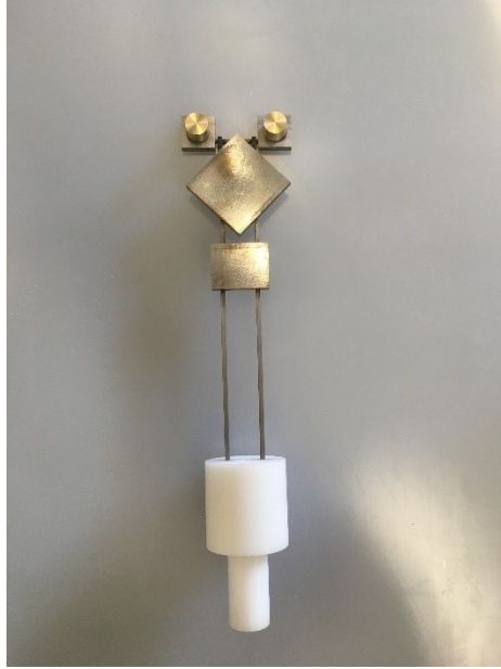
Figure 7.6 – Scale model of steel RICWS with plastic mount
