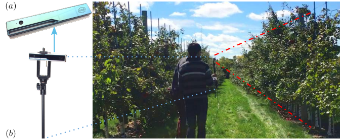
Fig. 1. Overview of data capturing scenario. (a): The RGB-D camera (Intel RealSense R200). (b): The RGB-D sensor is mounted on a stick to capture data from either horizontal view or titled top-down view.
