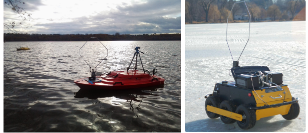
Fig. 2. Robotic systems for finding and tracking radio-tagged invasive fish.
