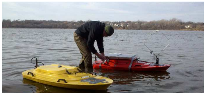
Figure 1: Two ASVs used in field experiments. The solar panels and tracking equipment are installed on the boat that acts as the searcher.
