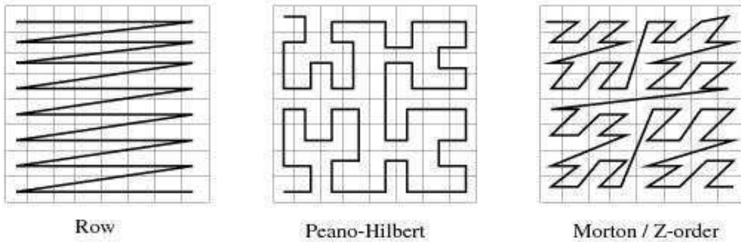
Figure 10: Space-filling curves to linearize a multidimensional space
