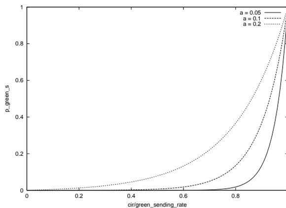
Figure 12: Marking probability function based on instantaneous green sending rate
