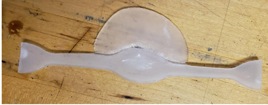
Figure 45: Sample obtained from center injection with the outer metal frame
