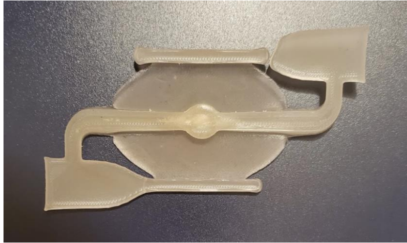
Figure 34: Run # 2 sample from DOE #2 showing the leakage of material from the runner
