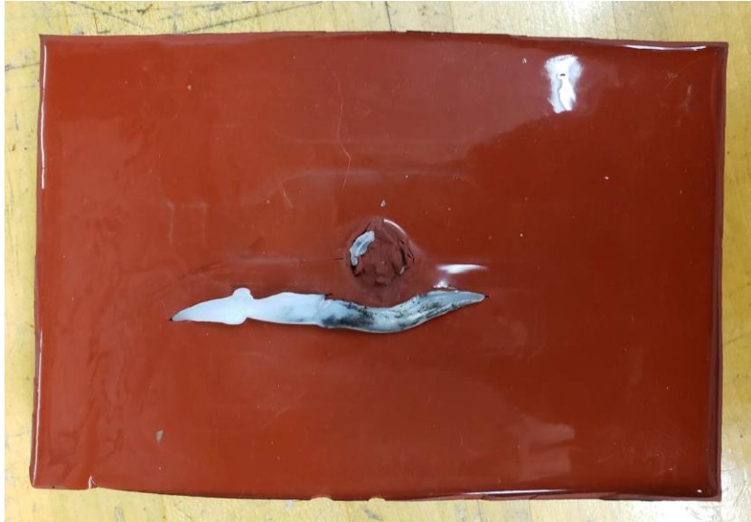
Figure 30: Bottom of the Durometer 60 mold tool. The PP material can be seen leaking to the bottom of the mold due to crack formation
