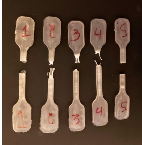
Figure 51: Metal mold samples after tensile testing
