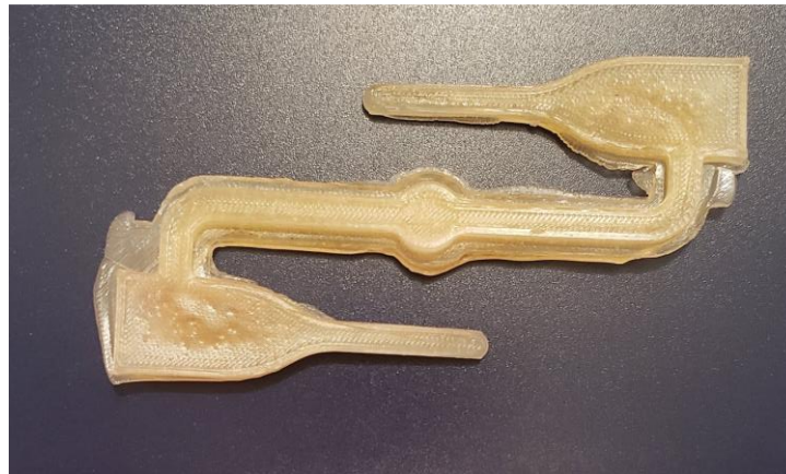
Figure 43: Sample obtained from 3D printed Nylon insert mold tool
