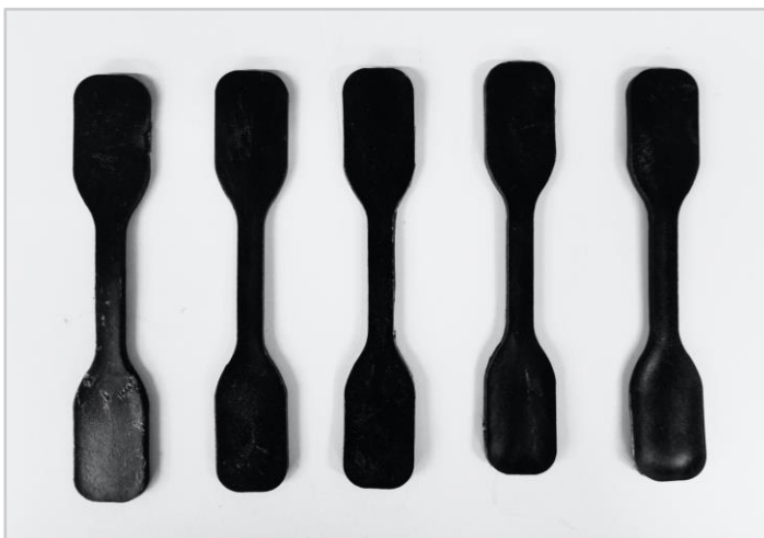
Figure 18: PP blended with lignin samples showing no sink marks
