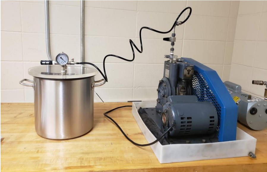
Figure 3: Equipment used for vacuum degassing of the silicone before pouring into the cast
