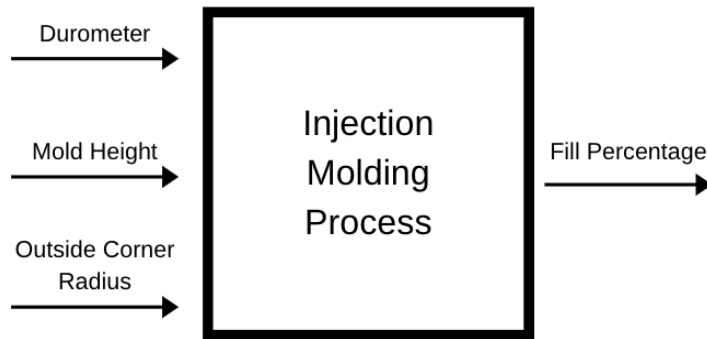
Figure 21: Injection molding process diagram for DOE #1
