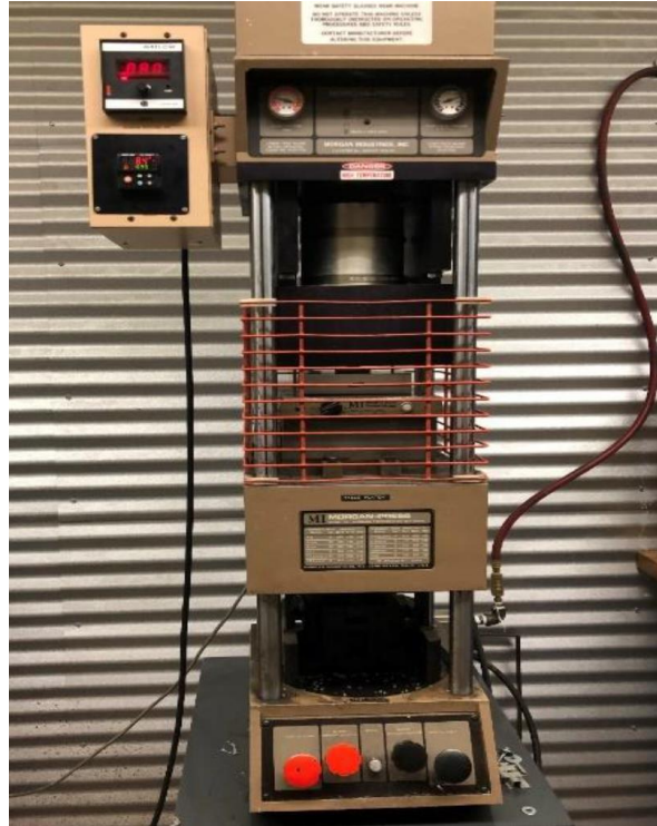
Figure 9: Morgan Press G-125T injection molding machine used in the experiments
