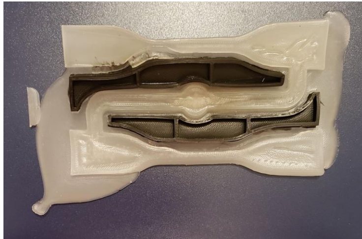
Figure 40: Sample showing 3D printed PLA insert melted with PP after solidifying
