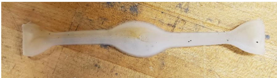
Figure 48: Sample obtained with center injection without outer frame
