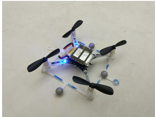
Figure 7.1: The physical platform (Crazyflie 2.0) experiments are performed with.
