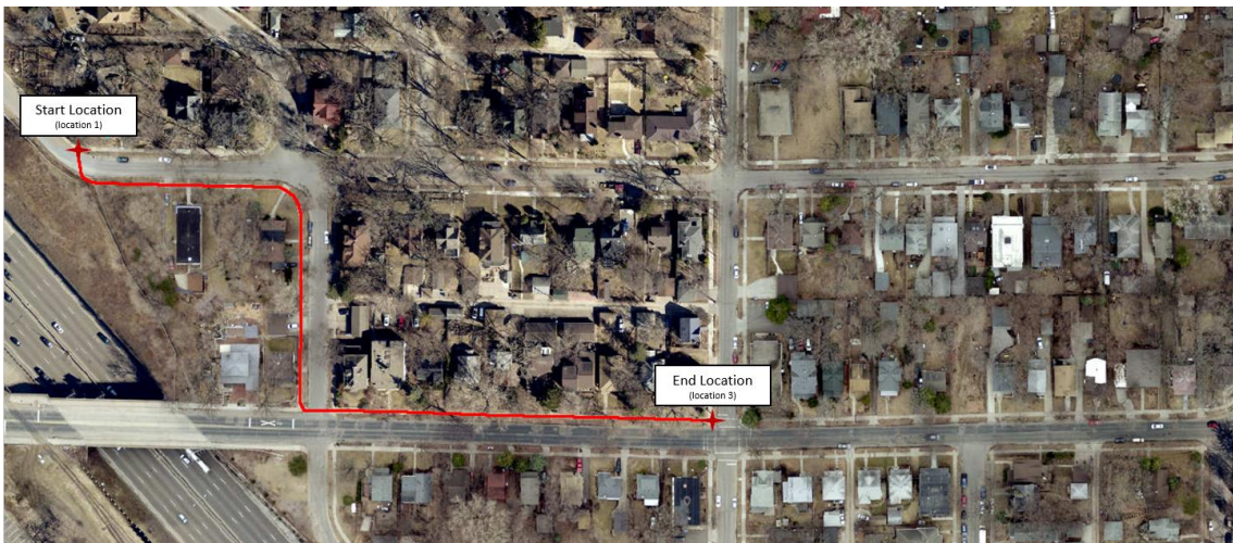
Figure 28- Path of the vehicle (red) traveling between two locations in the neighborhood without any active GNSS input to the EKF.
