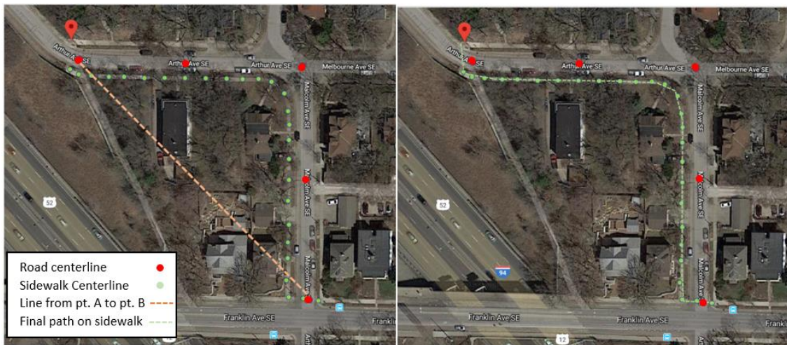
Figure 19- Line drawn between pt. A and pt. B assisting in path generation (left). The GNSS road centerlines (from Google Maps API) are shifted to the sidewalk (right).
