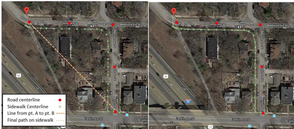
Figure 19. This line helps us pick one side of the street to favor over the other (if needed). The distances between all the possible sidewalk centerline nodes and the line drawn between pt. A and pt. B are calculated and the sum of these distances for the different path options are found. The set of sidewalk centerlines that are closest to the line provide a single solution for the path
