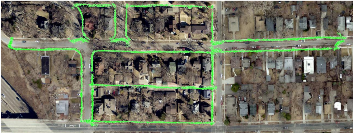
Figure 22- 2D pointcloud of segmented sidewalk overlaid on the orthorectified image.
