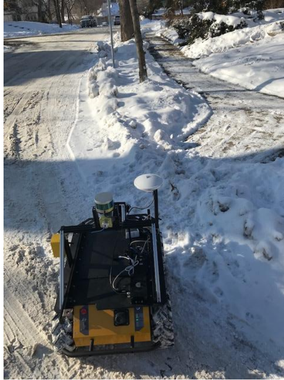
Figure 29- The vehicle encountering a pile of snow it is not able to travel through on a curbcut. The shadows show the difficulty traditional computer vision would encounter in urban neighborhoods.
