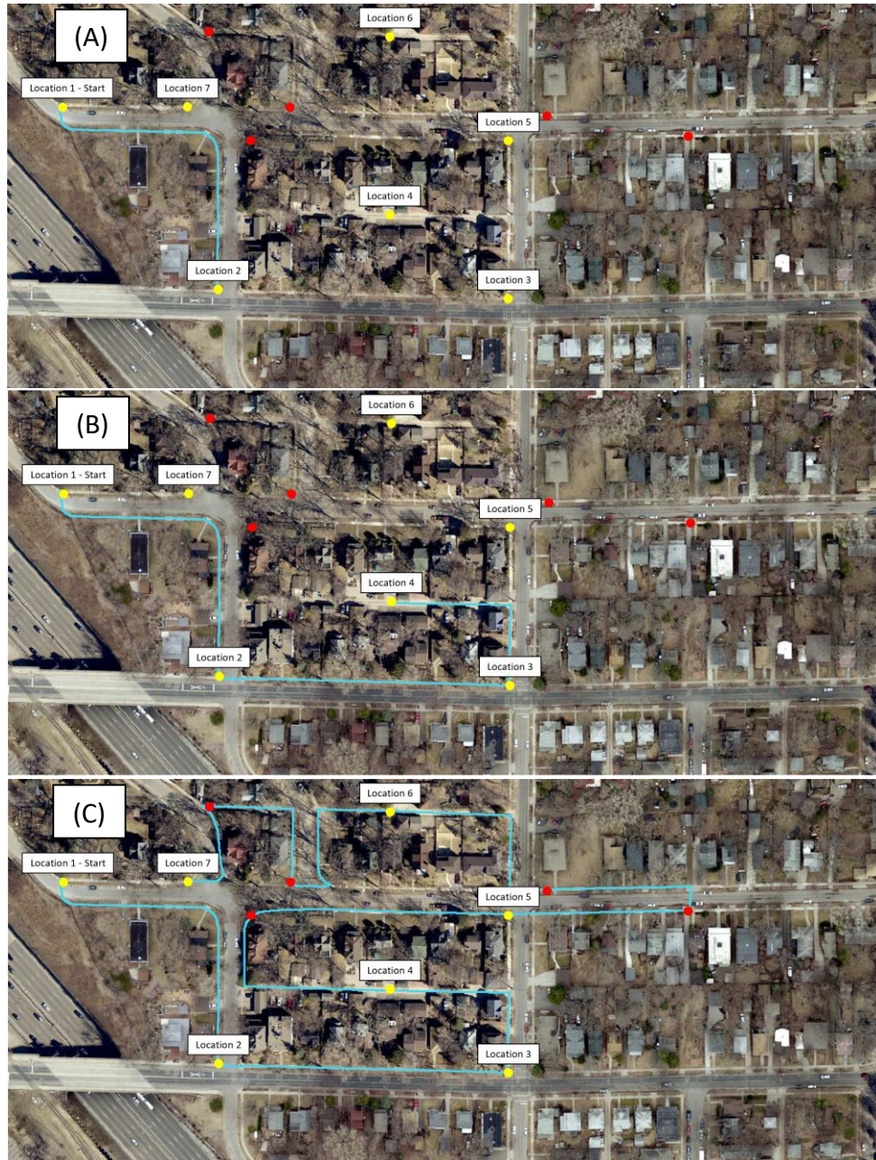
Figure 26- The paths taken by the vehicle between indicated locations shown in light blue. High accuracy GNSS locations shown as yellow circles and intermediate waypoints shown as red circles. (A) The path taken between location 1 and location 2. (B) The path taken between location 1 and location 4 (traveling through locations 2 and 3). (C) The path taken between location 1 and location 7.
