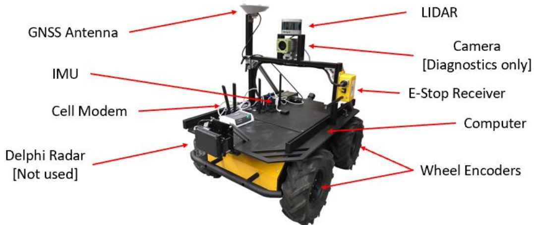
Figure 2 – The hardware and sensors mounted on the Husky platform that are used for this research.
