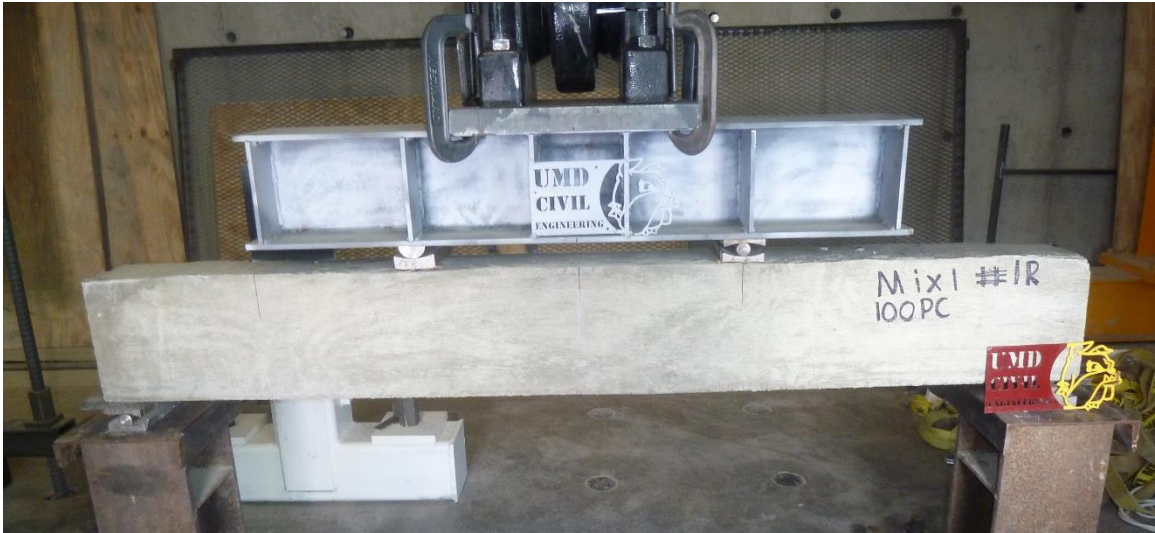
Figure C.1. Mixture 1 (100PC) beam #1R: concrete beam before testing.
