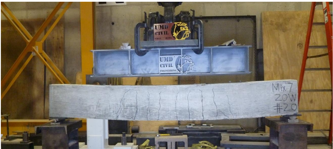
Figure C.40. Mixture 7 (20W) beam #20: concrete beam after testing.
