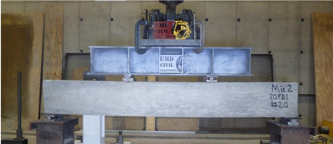
Figure C.9. Mixture 2 (20FA1) beam #20: concrete beam before testing.
