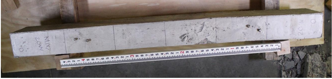
Figure D.61. Mixture 7 (20W) beam #30: concrete beam top view.
