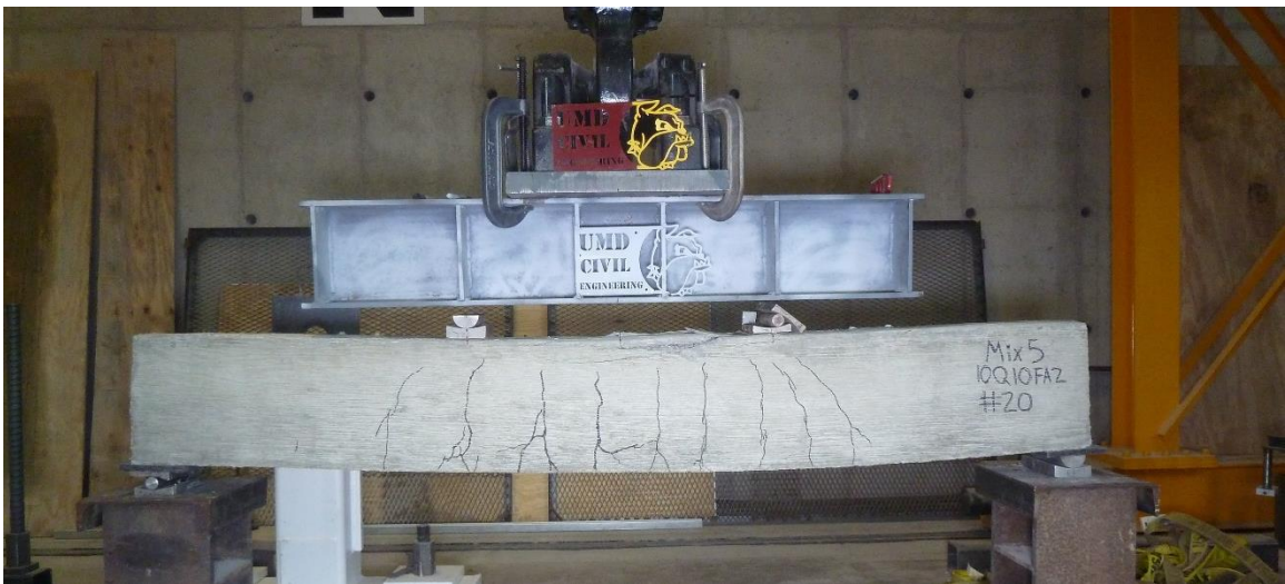
Figure C.28. Mixture 5 (10Q10FA2) beam #20: concrete beam after testing.
