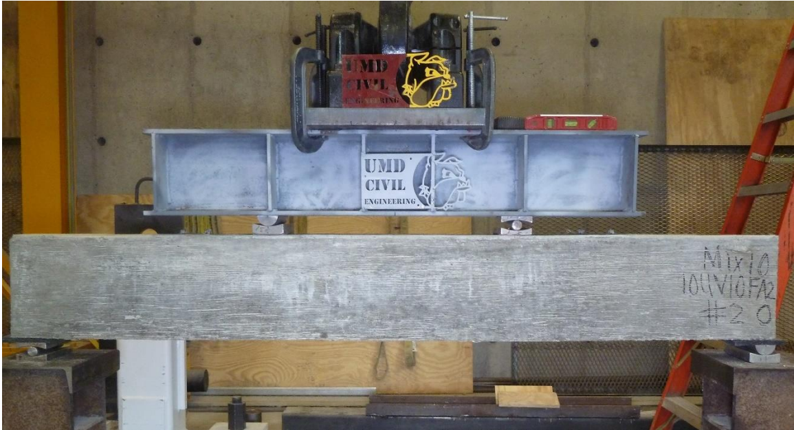
Figure C.57. Mixture 10 (10UV10FA2) beam #20: concrete beam before testing.
