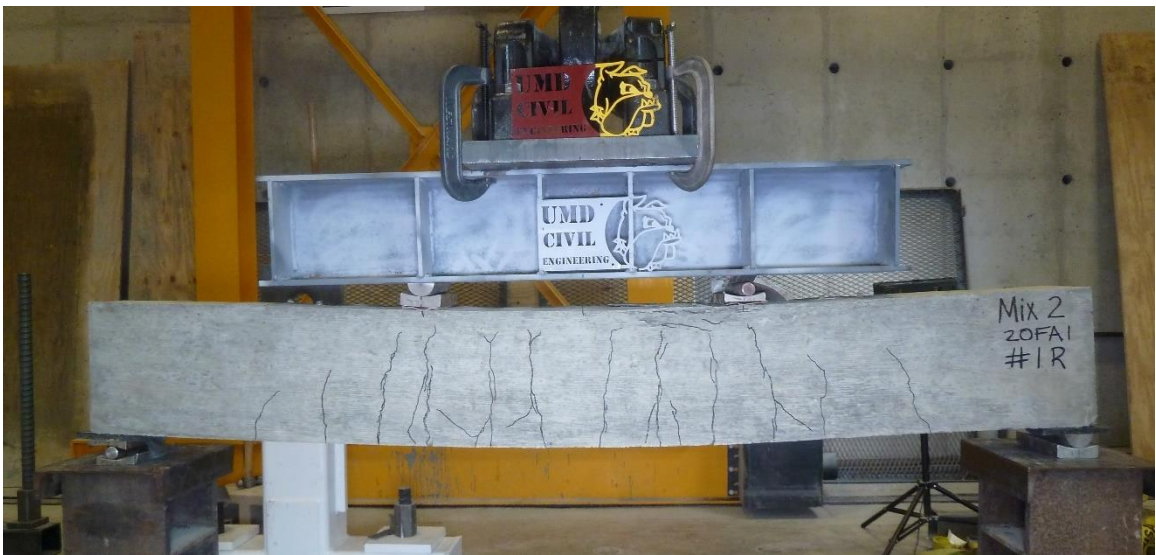
Figure C.8. Mixture 2 (20FA1) beam #1R: concrete beam after testing.
