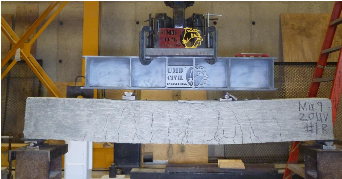
Figure C.50. Mixture 8 (20UV) beam #1R: concrete beam after testing.
