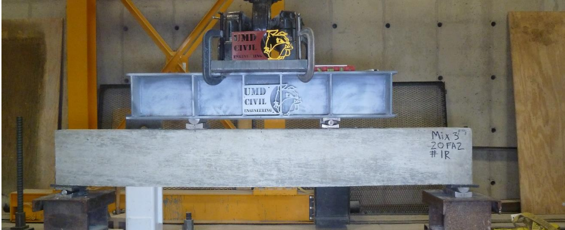
Figure C.13. Mixture 3 (20FA2) beam #1R: concrete beam before testing.
