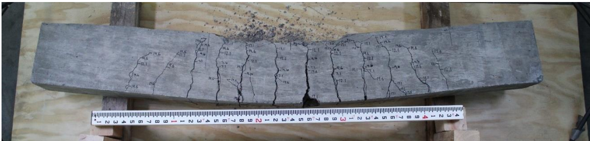
Figure D.2. Mixture 1 (100PC) beam #1R: concrete beam side view.
