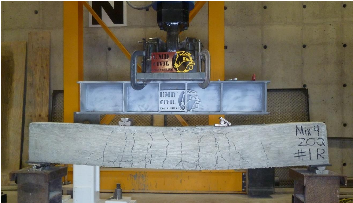
Figure C.20. Mixture 4 (20Q) beam #1R: concrete beam after testing.
