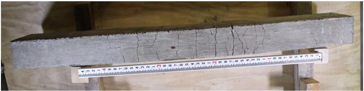
Figure D.69. Mixture 8 (10W10FA1) beam #20: concrete beam bottom view.
