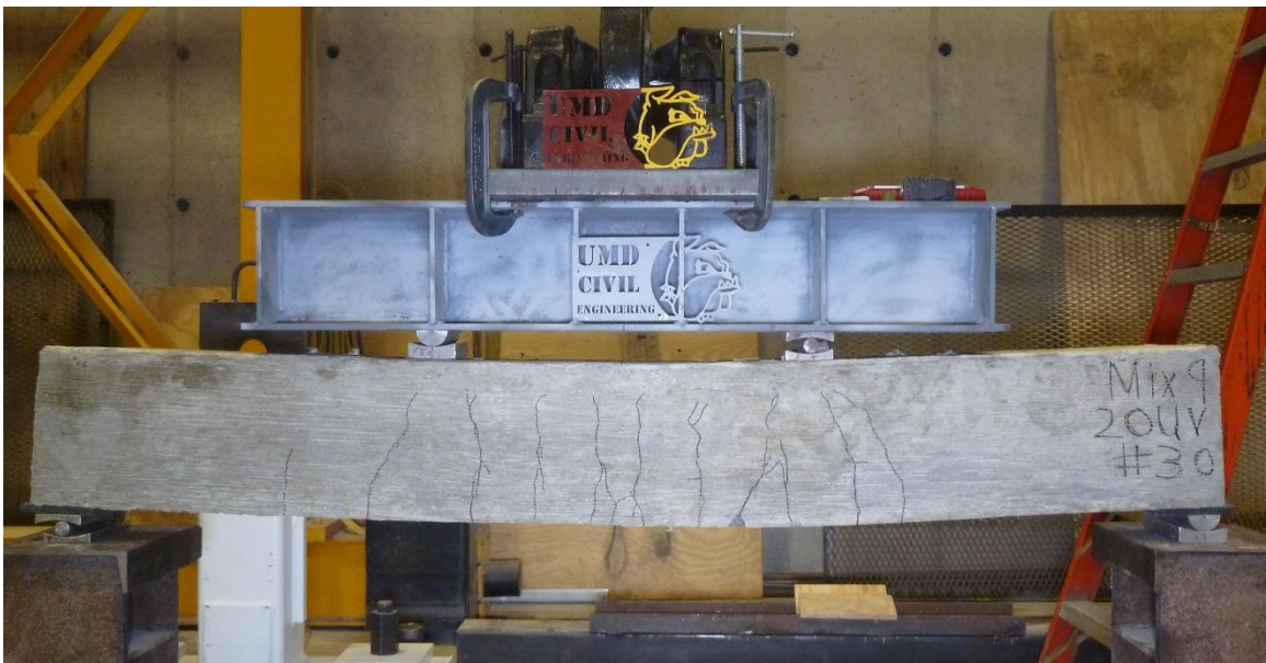
Figure C.54. Mixture 8 (20UV) beam #30: concrete beam after testing.
