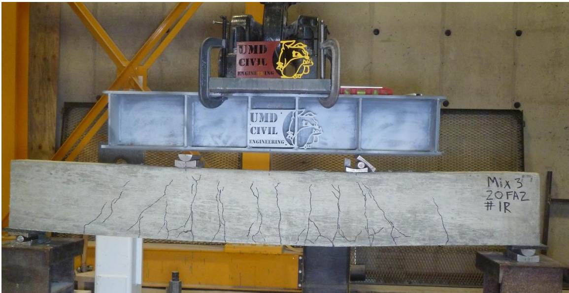
Figure C.14. Mixture 3 (20FA2) beam #1R: concrete beam after testing.
