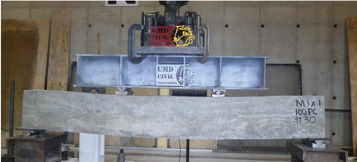
Figure C.5. Mixture 1 (100PC) beam #30: concrete beam before testing.
