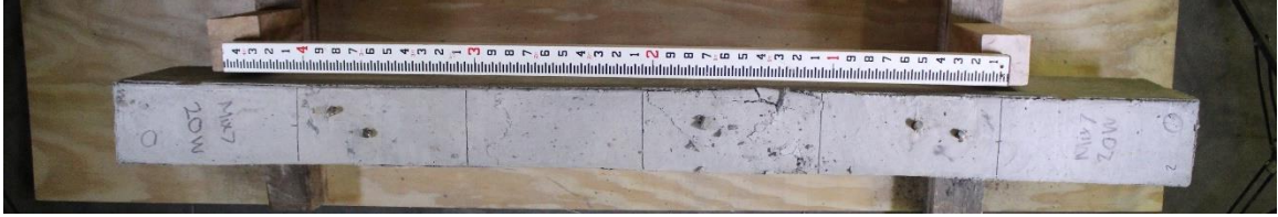
Figure D.58. Mixture 7 (20W) beam #20: concrete beam top view.
