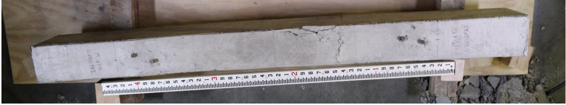
Figure D.85. Mixture 10 (10UV10FA2) beam #20: concrete beam top view.
