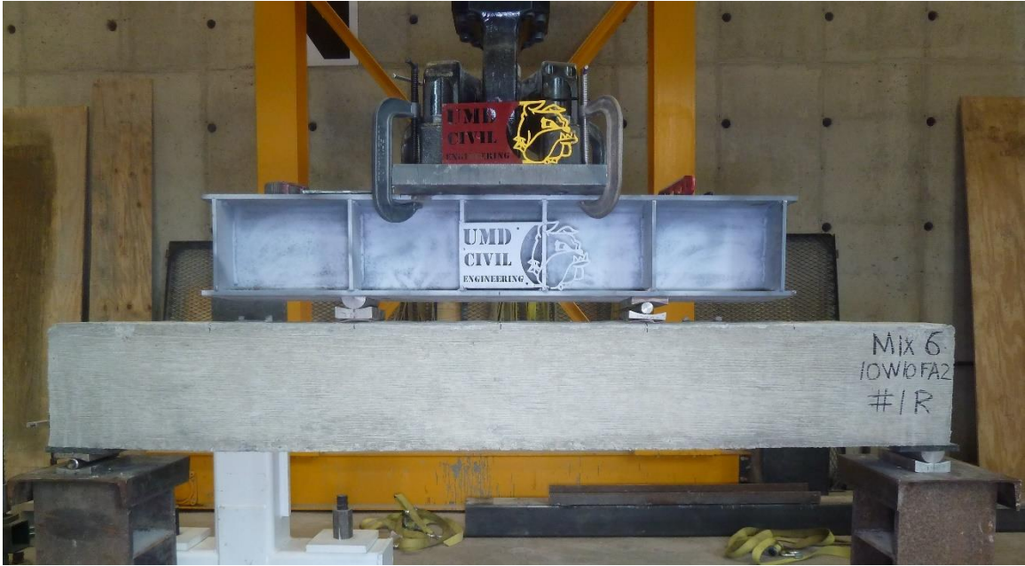
Figure C.31. Mixture 6 (10W10FA2) beam #1R: concrete beam before testing.
