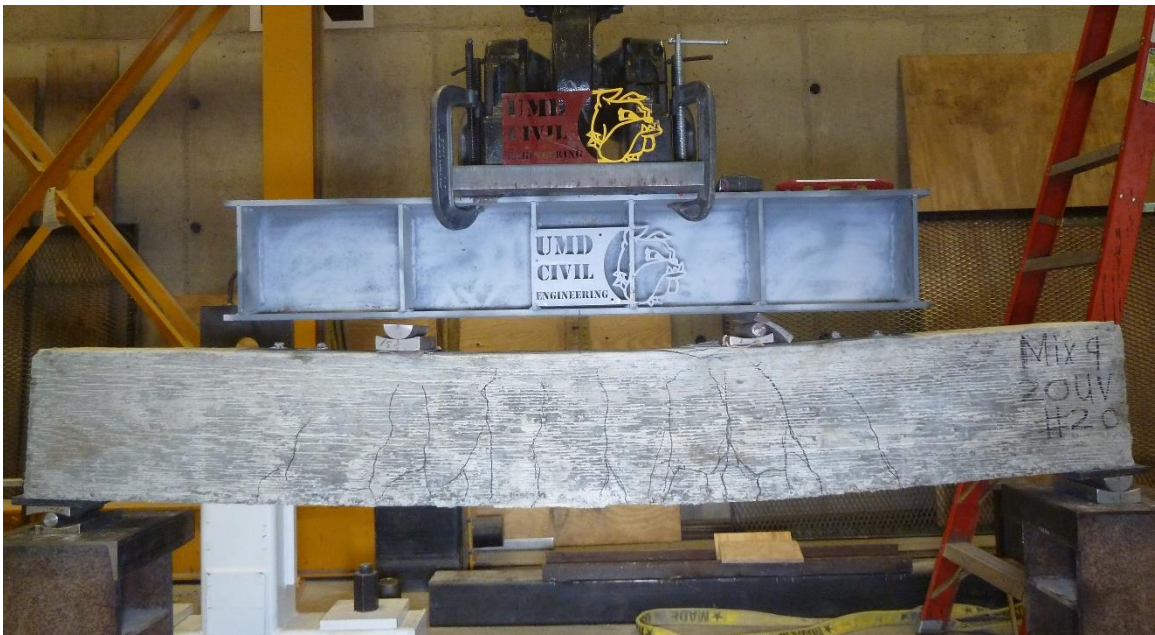
Figure C.52. Mixture 8 (20UV) beam #20: concrete beam after testing.
