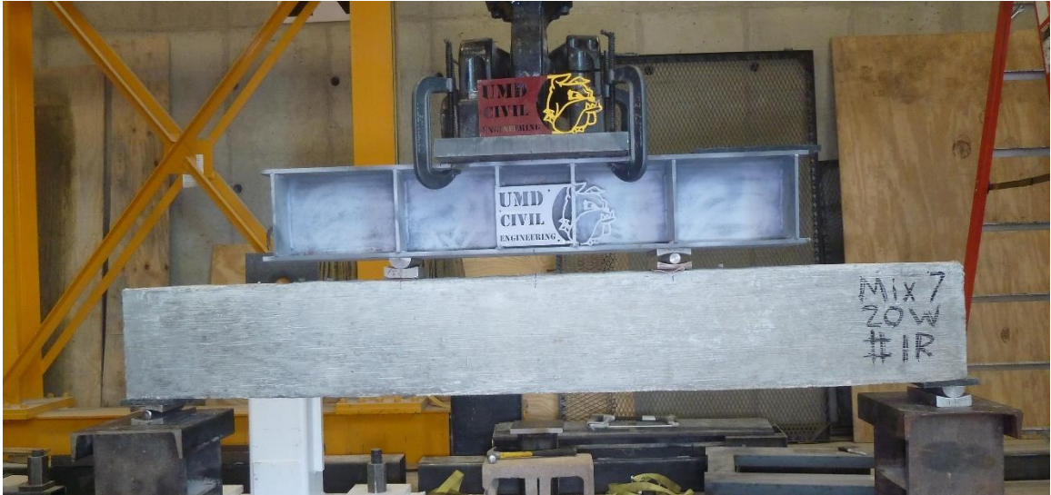
Figure C.37. Mixture 7 (20W) beam #1R: concrete beam before testing.
