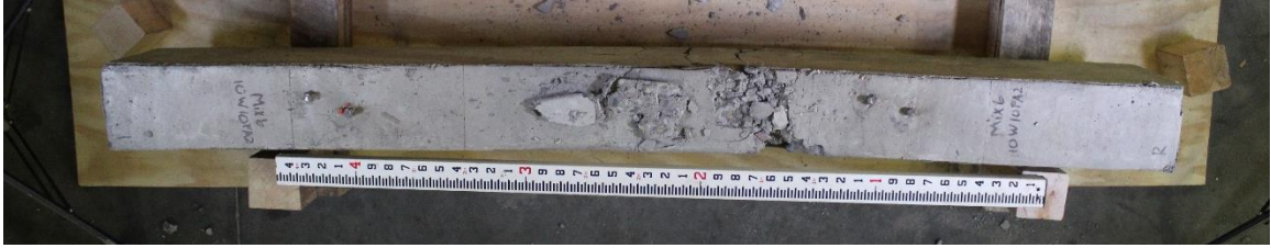
Figure D.46. Mixture 6 (10W10FA2) beam #1R: concrete beam top view.
