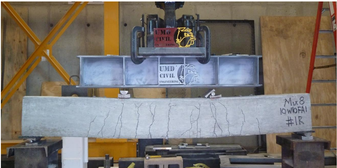
Figure C.44. Mixture 8 (10W10FA1) beam #1R: concrete beam after testing.
