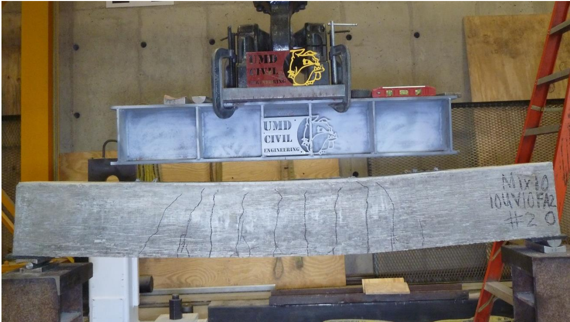
Figure C.58. Mixture 10 (10UV10FA2) beam #20: concrete beam after testing.
