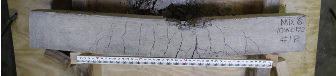
Figure D.47. Mixture 6 (10W10FA2) beam #1R: concrete beam side view.
