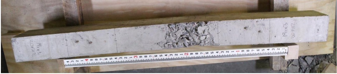
Figure D.25. Mixture 3 (20FA2) beam #30: concrete beam top view.
