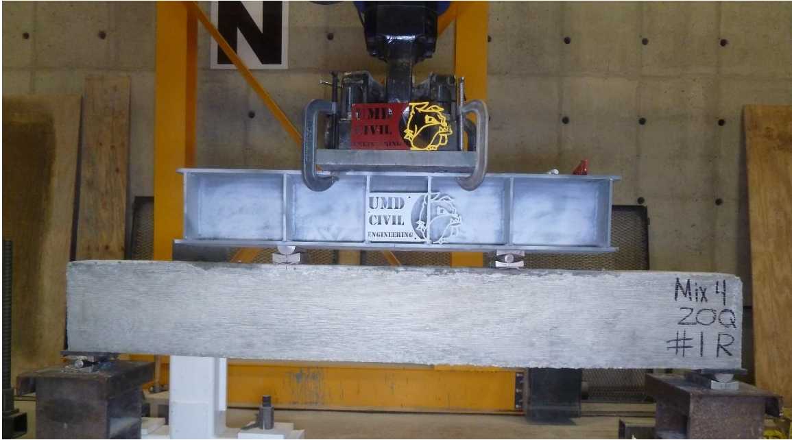
Figure C.19. Mixture 4 (20Q) beam #1R: concrete beam before testing.
