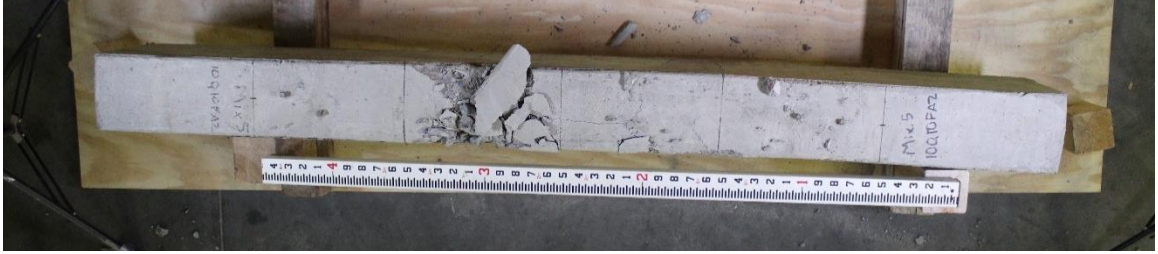
Figure D.43. Mixture 5 (10Q10FA2) beam #30: concrete beam top view.
