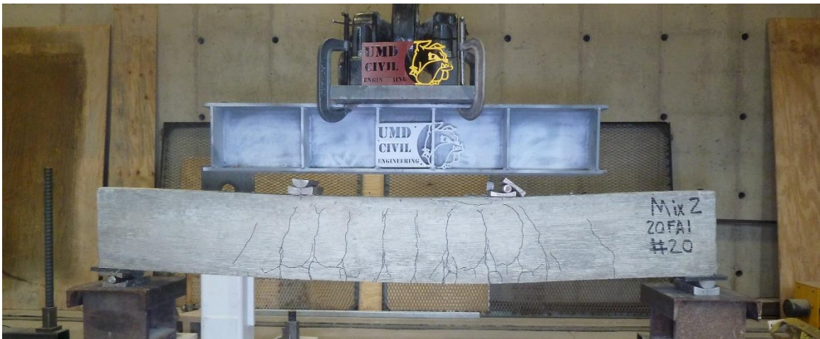
Figure C.10. Mixture 2 (20FA1) beam #20: concrete beam after testing.
