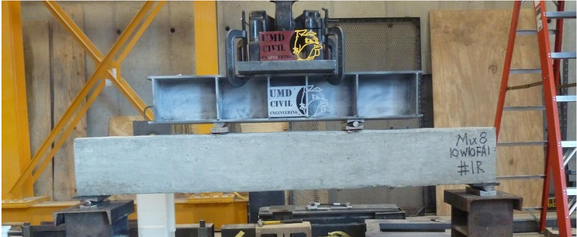
Figure C.43. Mixture 8 (10W10FA1) beam #1R: concrete beam before testing.
