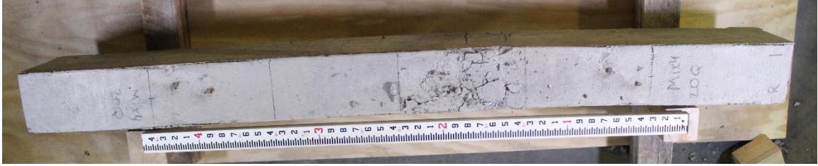
Figure D.28. Mixture 4 (20Q) beam #1R: concrete beam top view.
