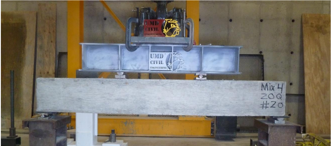
Figure C.21. Mixture 4 (20Q) beam #20: concrete beam before testing.
