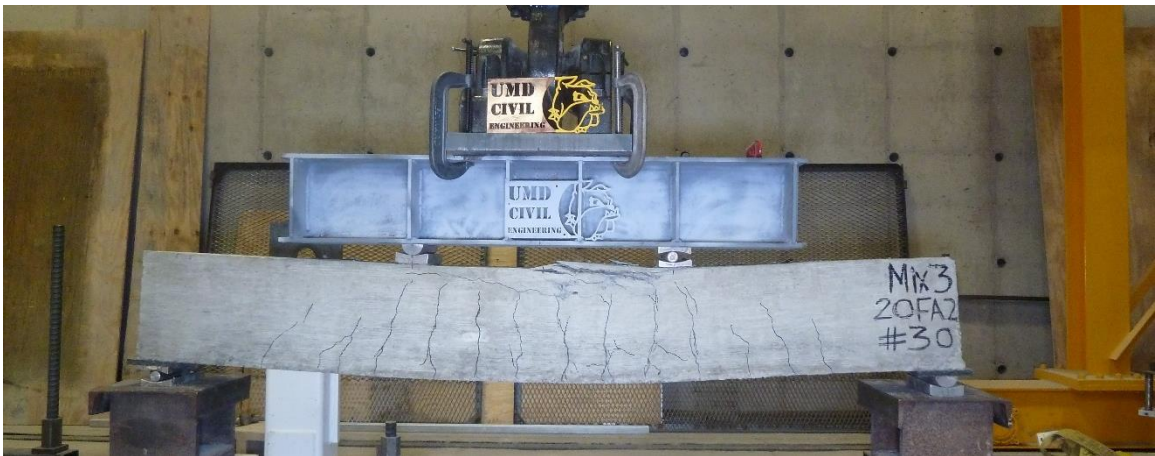
Figure C.18. Mixture 3 (20FA2) beam #30: concrete beam after testing.
