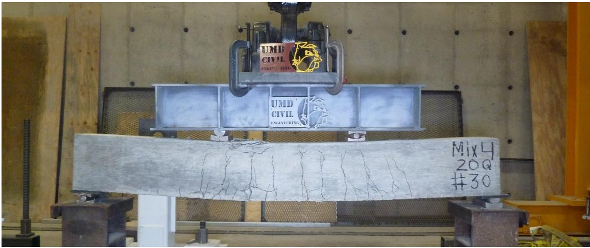
Figure C.24. Mixture 4 (20Q) beam #30: concrete beam after testing.
