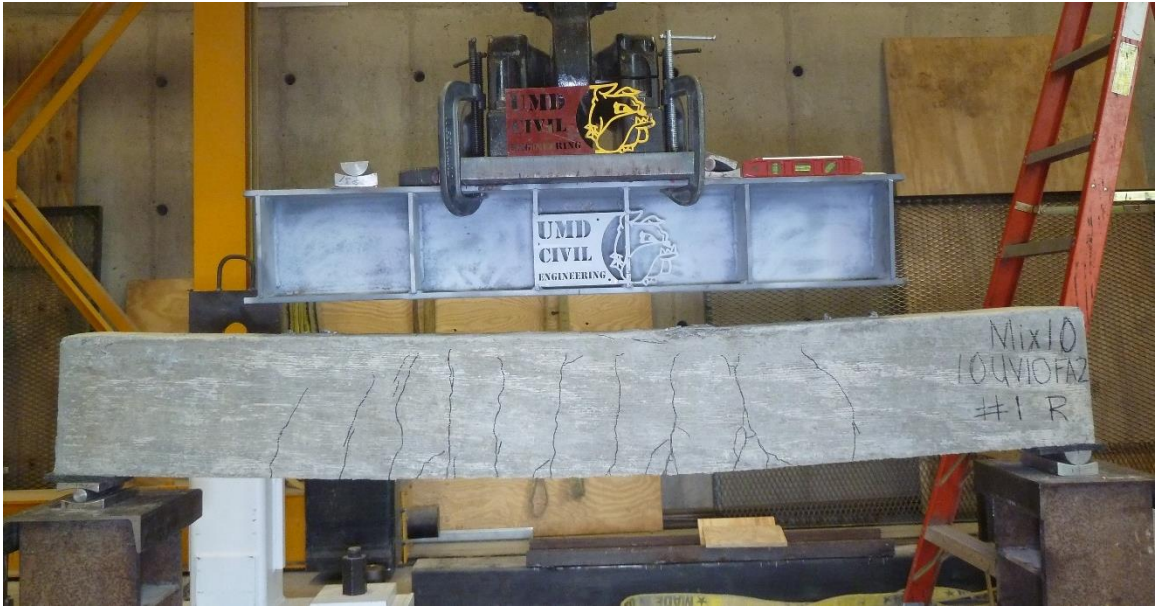
Figure C.56. Mixture 10 (10UV10FA2) beam #1R: concrete beam after testing.
