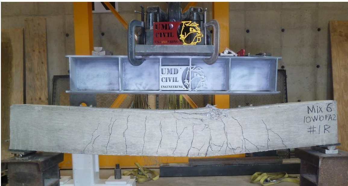
Figure C.32. Mixture 6 (10W10FA2) beam #1R: concrete beam after testing.
