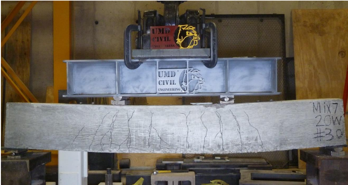
Figure C.42. Mixture 7 (20W) beam #30: concrete beam after testing.
