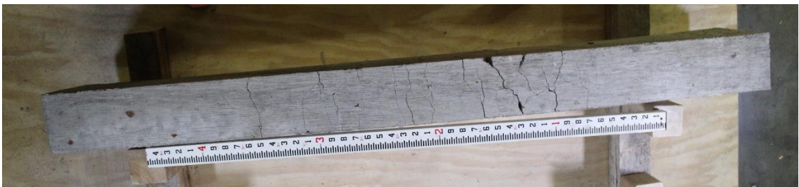
Figure D.84. Mixture 10 (10UV10FA2) beam #1R: concrete beam bottom view.
