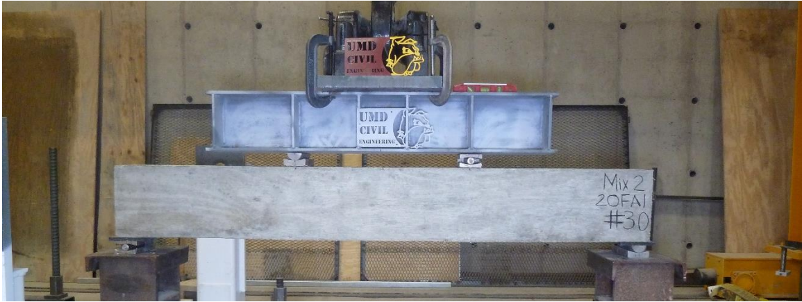
Figure C.11. Mixture 2 (20FA1) beam #30: concrete beam before testing.
