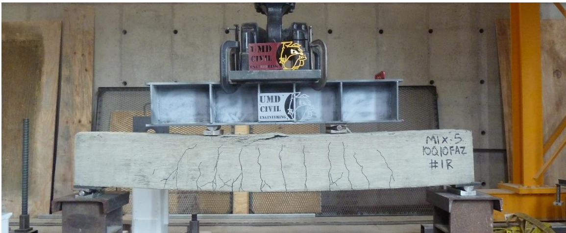
Figure C.26. Mixture 5 (10Q10FA2) beam #1R: concrete beam after testing.
