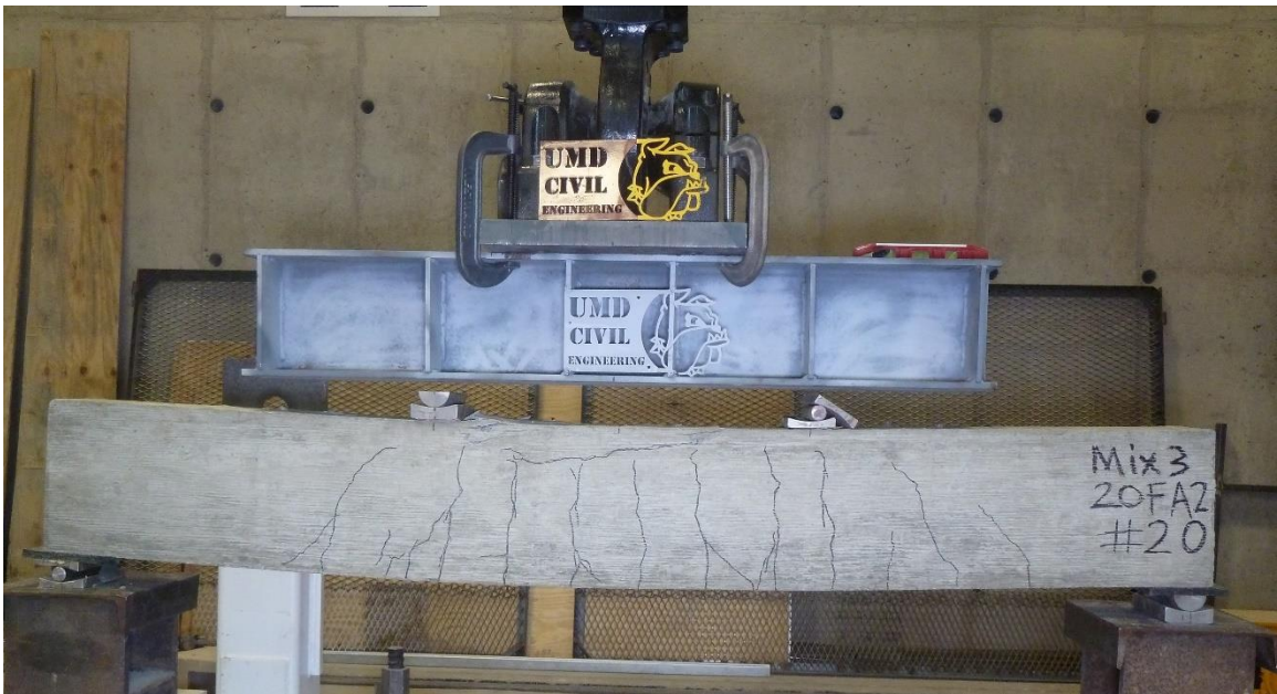
Figure C.16. Mixture 3 (20FA2) beam #20: concrete beam after testing.
