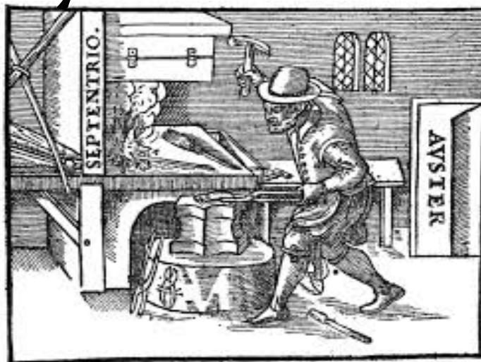
Fig. 1. A thermoremanent anisotropy experiment described by William Gilbert in 1600. When a red-hot iron spike is allowed to cool while pointing from the south (Auster) to the north (Septentrio), it acquires a strong remanence. Cooling in the east-west orientation, with the long axis perpendicular to the ambient field, produces a much weaker TRM.
