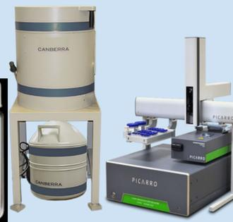
Figure 6: Gamma Counter for  $^{210}\text{Pb}$  and  $^7\text{Be}$
