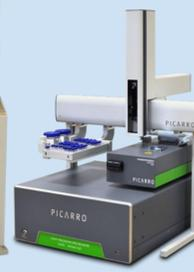
Figure 7: Isotope and Gas Concentration Analyzer
