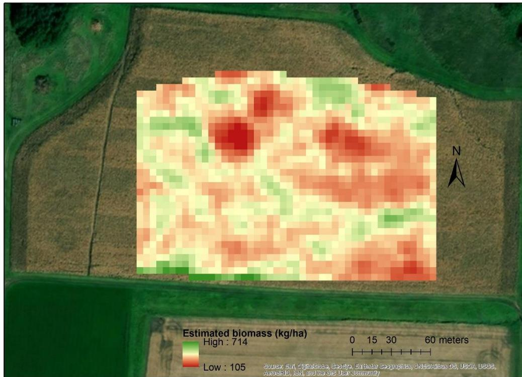
Figure 4.5. Spatial variability in maize biomass at the five leaf-collar stage estimated using NDVI values from RapidEye satellite imagery.
