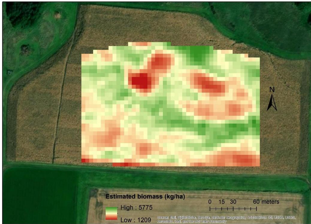
Figure 4.6. Spatial variability in maize biomass at ten-leaf collar stage estimated using NDVI values from RapidEye satellite image.
