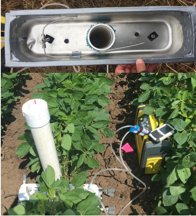
Figure 3.2 Images of the inside of the chamber (top) and the chamber deployed in the field (bottom).
