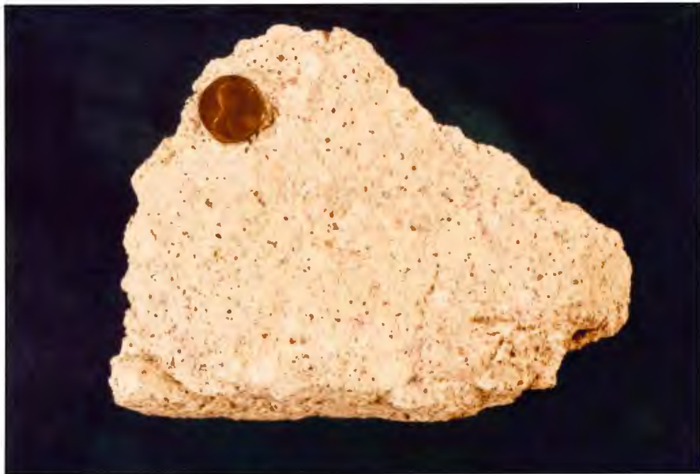
Figure 28: Handsample of the crystal vitric tuff of Unit II of the Goldens Ranch Formation taken from an exposure in the Painted Rocks area. White spots are pumice, dark flecks are biotite. (Photo courtesy of S. R. Osterberg.)
