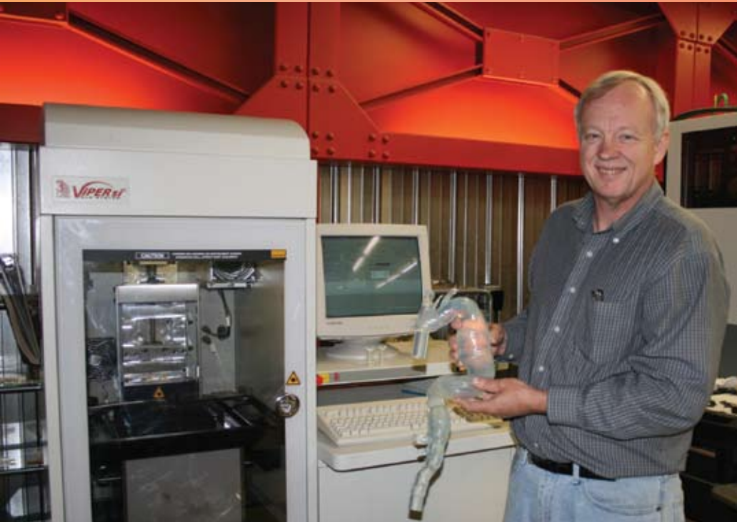
Prototype lab director Steve Kossett uses stereolithography to make a model used to improve medical stents.
