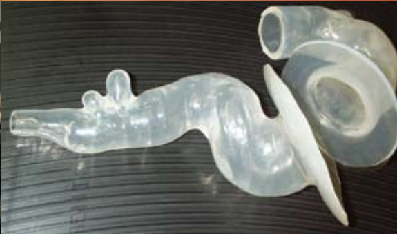
Prototype lab director Steve Kossett uses stereolithography to make a model used to improve medical stents.
