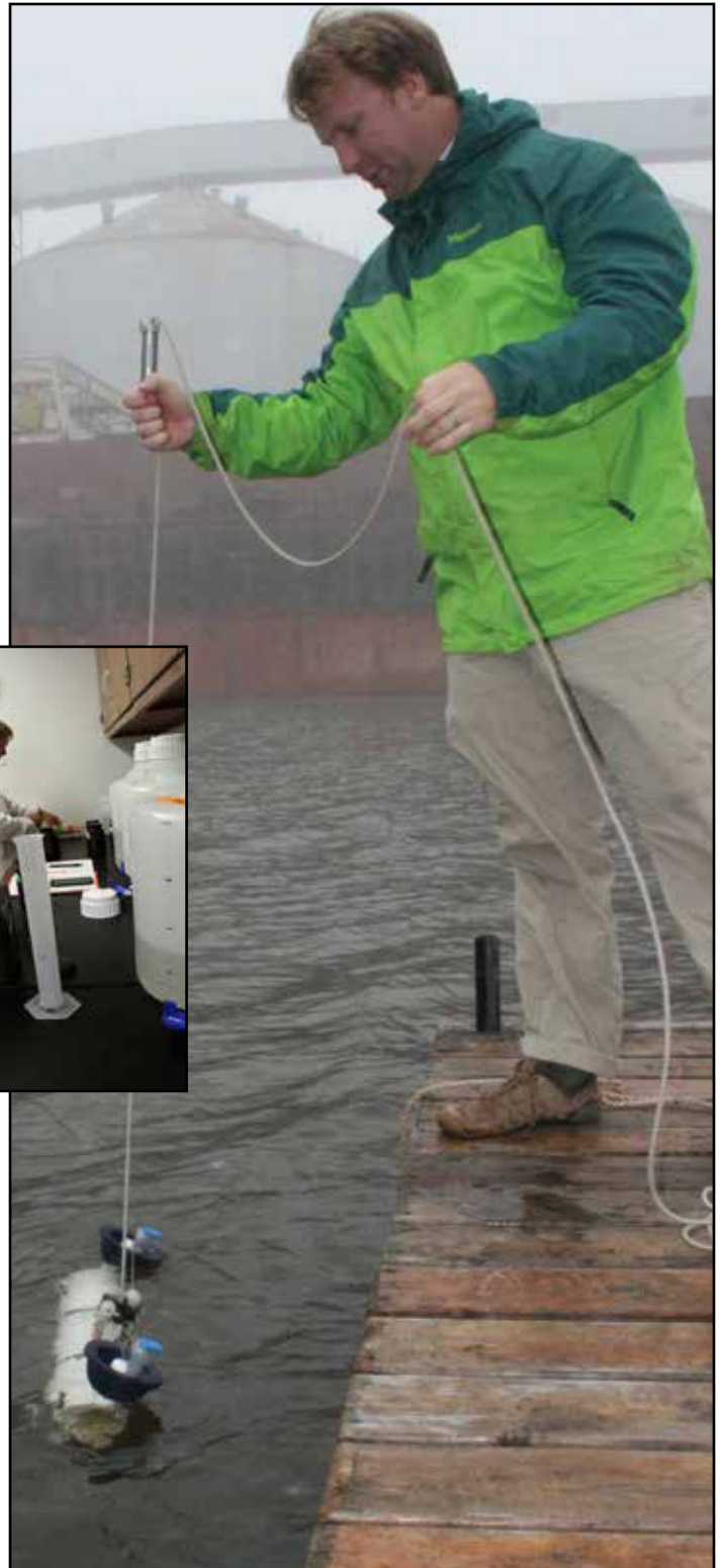
NRRI scientist Andrew Bramburger lowers a sampler into the harbor to collect water for testing in the lab. (Inset) Euan Reavie pours water into tubes.
