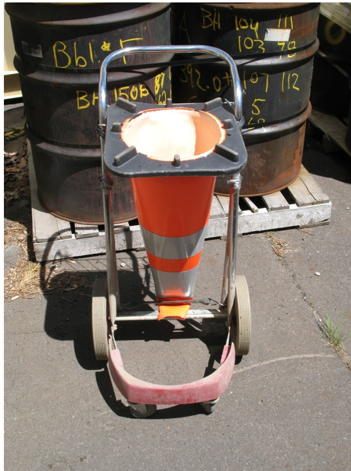
Figure 2.6 Inverted cone apparatus used by the NRRRI for May 24, 2017, test.
