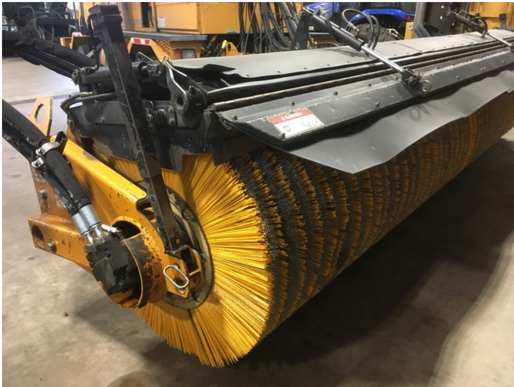
Figure 2.100 Brush end of airport runway sweeper.
