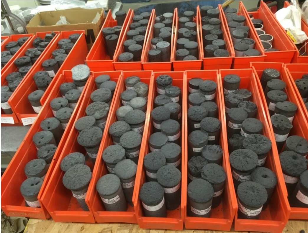
Figure 2.37 Some of the 2" diameter x 4" tall cylinder specimens prepared during formulation development.
