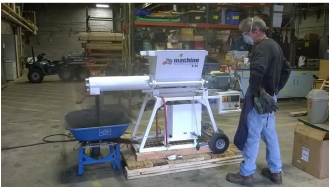
Figure 2.23 Testing throughput of dry reactive aggregate in continuous mixing device, October 5, 2017.
