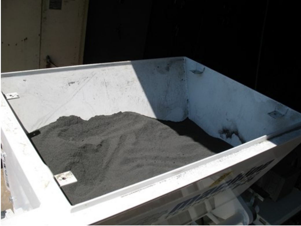
Figure 2.18 Continuous mixer hopper filled with reactive aggregate.
