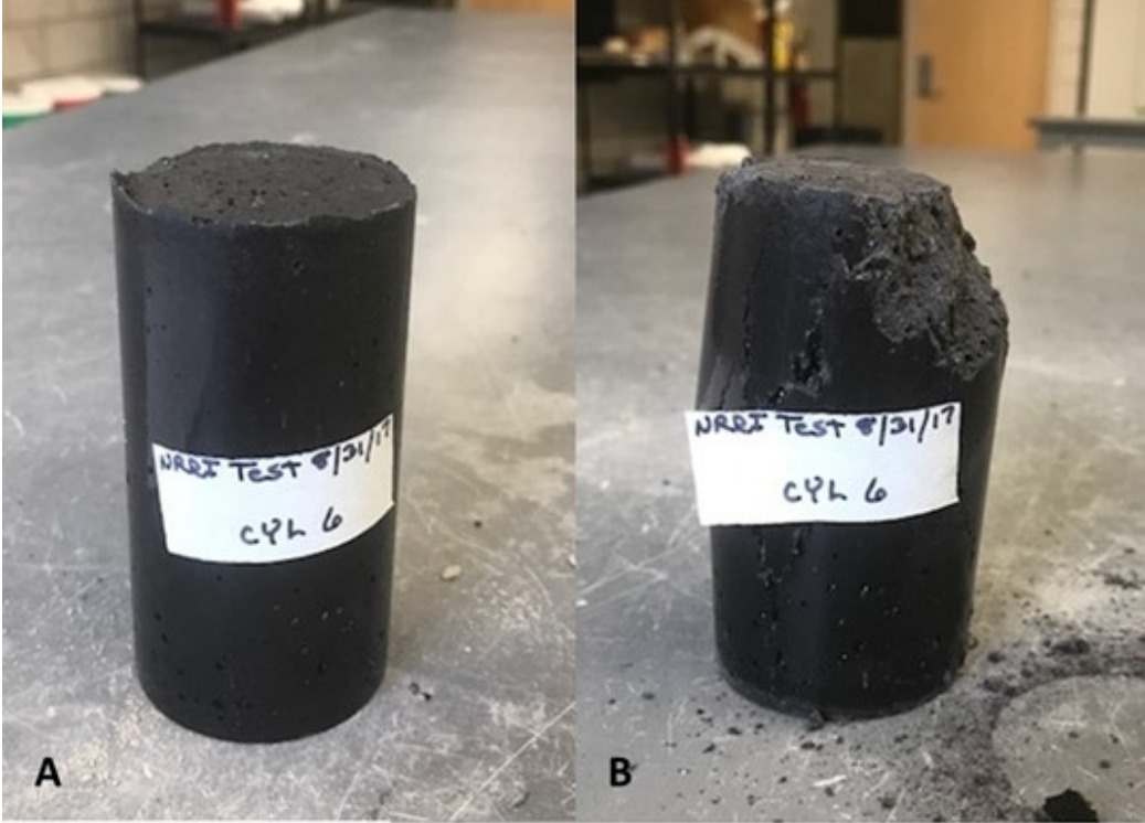
Figure 2.20 2" x 4" test cylinders, before (A) and after (B) uniaxial compressive strength testing.
