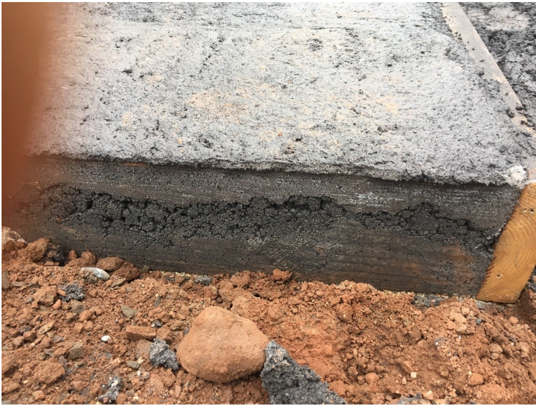
Figure 2.12 Sidewalk slab made from fine formulation (October 2016).
