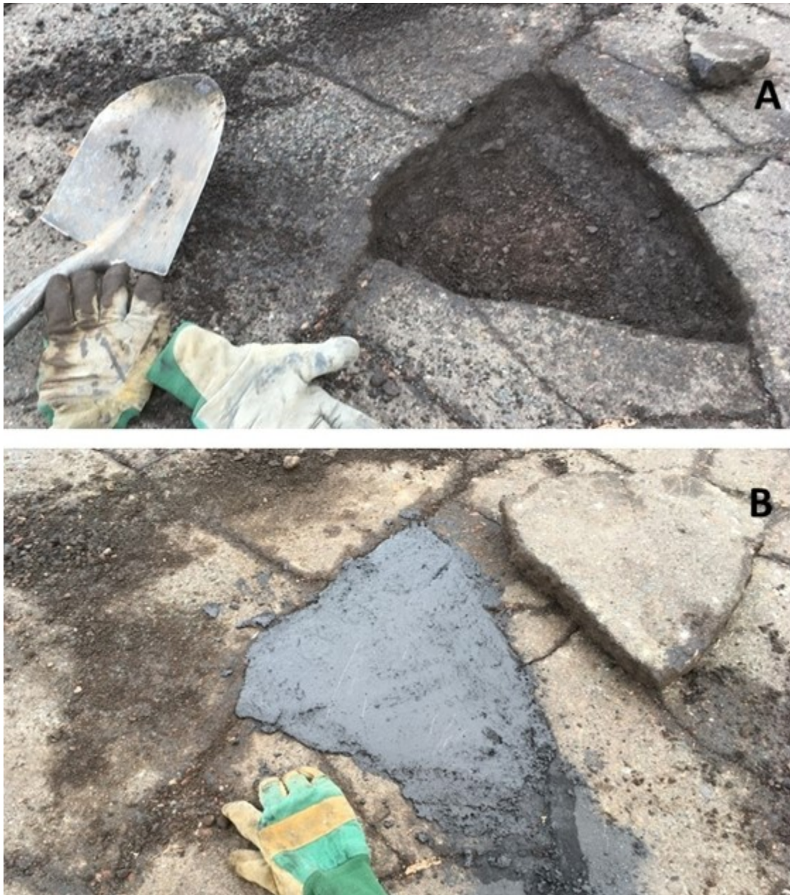
Figure 2.36 November 20, 2017, cold temperature pothole test at NRRRI; before (A) and after (B).
