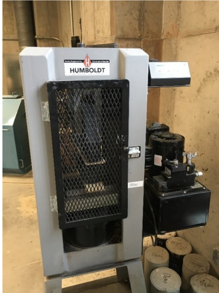
Figure A1. Test Set-up: split tensile strength.
