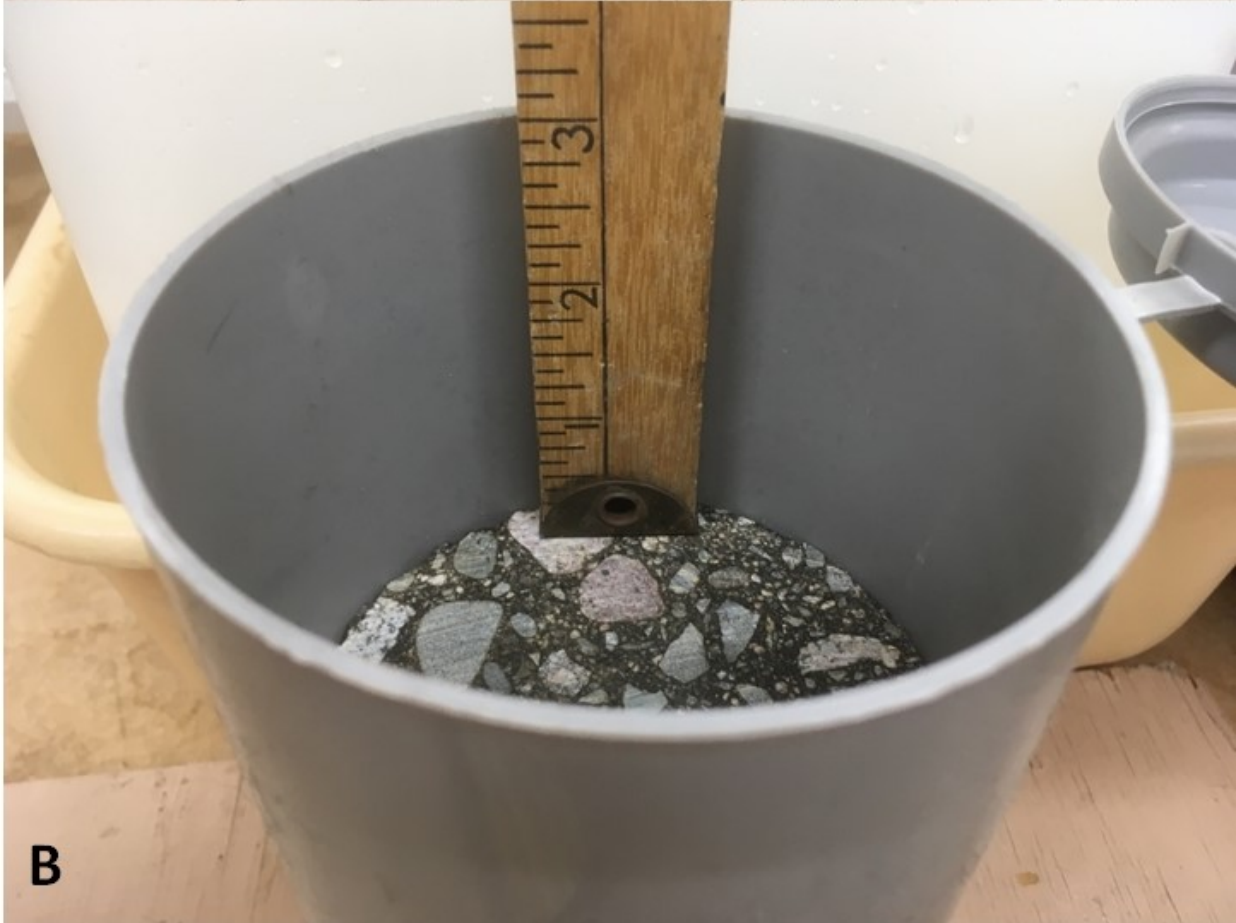
Figure 2.54 Asphalt pavement core sawed to 3" thick (A) and placed in 4" diameter cylinder (B).
