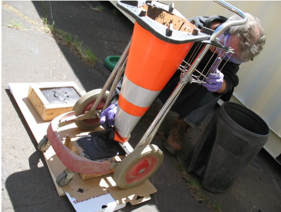
Figure 2.9 Filling of “pothole” forms (May 24, 2017).
