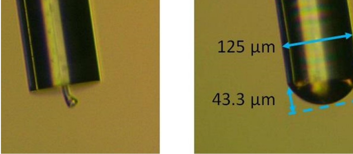
Figure 4.6: Microscope images of the device (a) after fabrication of the wave-guiding pillar and (b) after the dip-coating of the surrounding epoxy.
