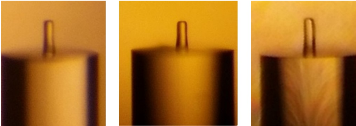
Figure 4.13: Photographs of straight pillars obtained using 405-nm curing and multiple samples demonstrate repeatability of the process. Fiber diameter is 125\ \mu\text{m} , and pillar diameter is 9\ \mu\text{m} .
