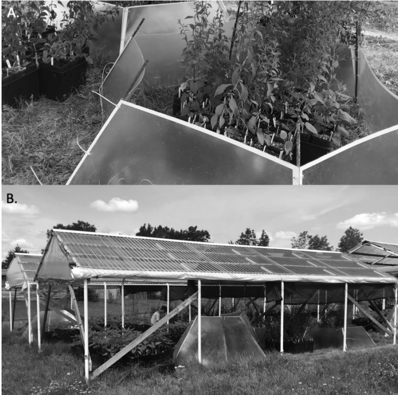
Figure 2.2. Photos of the A) elevated temperature chambers and B) rainout shelters, used to impose/control the temperature and water treatments in this study.
