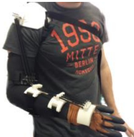
Figure 7: Bowden cable SMA elbow bend exoskeleton by Copaci et. al.
