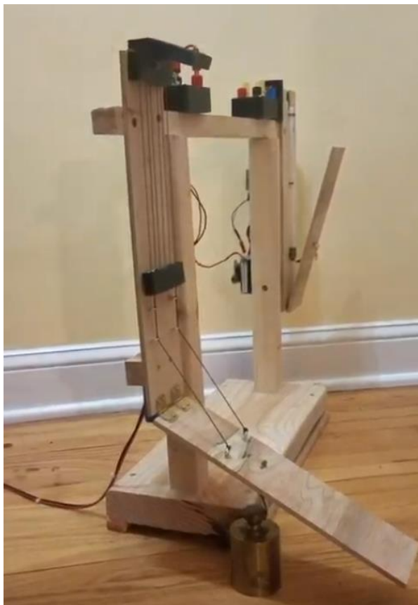
Figure 41: Arm rig with extensional strain of 1.5 with a 1 kg weight.
