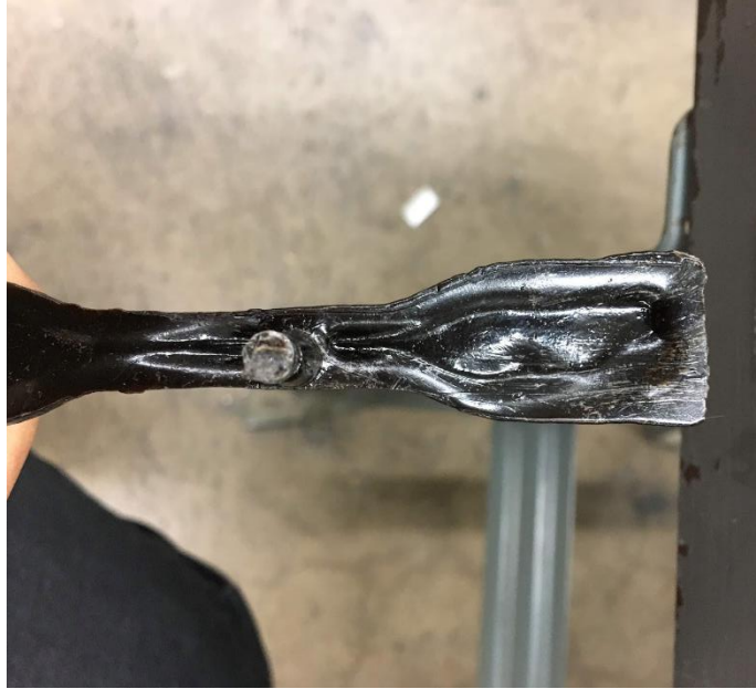
Figure 3. 6 Sink mark in injected sample
