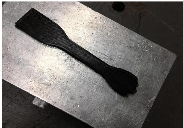
Figure 3. 5 Incomplete injection with lignin
