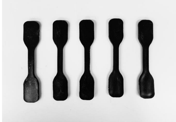
Figure 4. 1 HDPE-lignin ASTM D638 Type IV tensile test coupons
