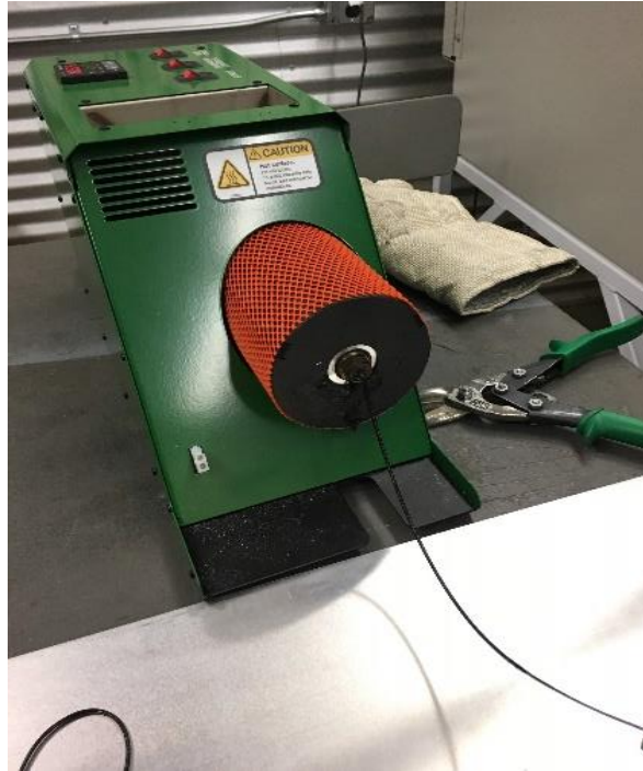
Figure 3. 3 Processing blend filaments with Filabot EX2 single screw extruder
